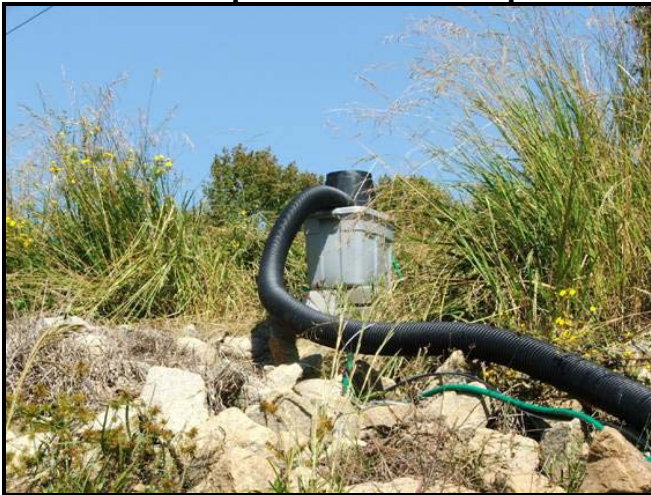
Photo 1: Experimental Eel Ramp Located at the Tailrace of the Saluda Hydro Project
