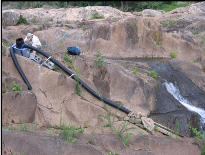
Photo 3: Experimental Eel Ramp Located at the Spillway of the Saluda Hydro Project
