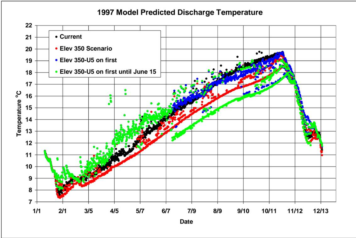
Figure 4-50. 1997 Release Temperature
