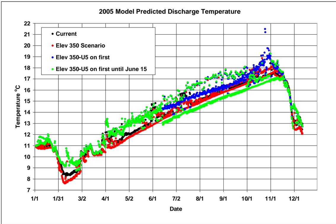
Figure 4-58. 2005 Release Temperature
