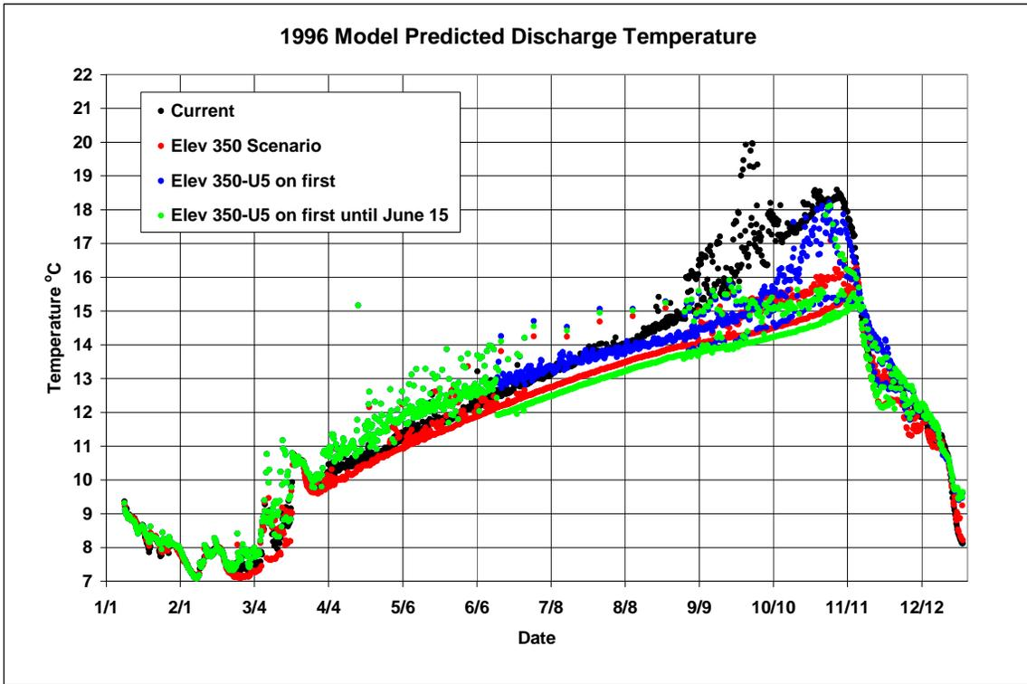
Figure 4-48. 1996 Release Temperature
