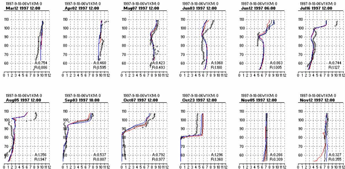
**Figure 6-51. 1997 Modeled and Observed DO Profiles in the Forebay of Lake Murray; Overall Statistics: ABS = 0.73, RMS = 1.02**
