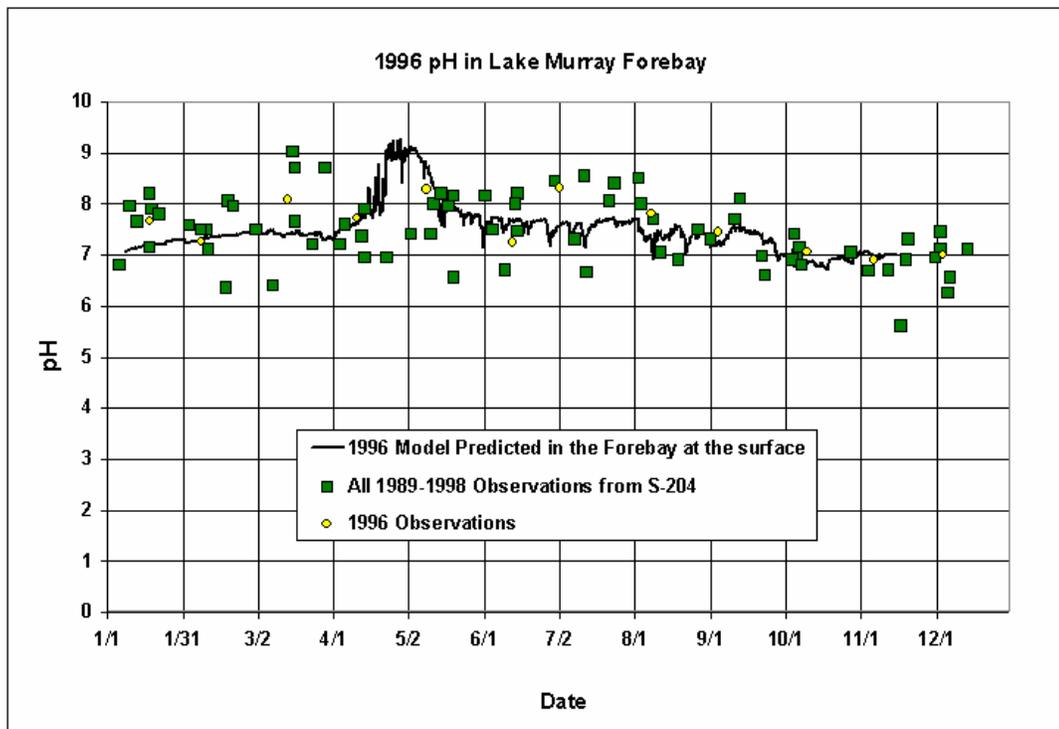
**Figure 6-65. 1996 Comparison of Modeled Derived versus Measured pH at the Surface in the Forebay of Lake Murray**
