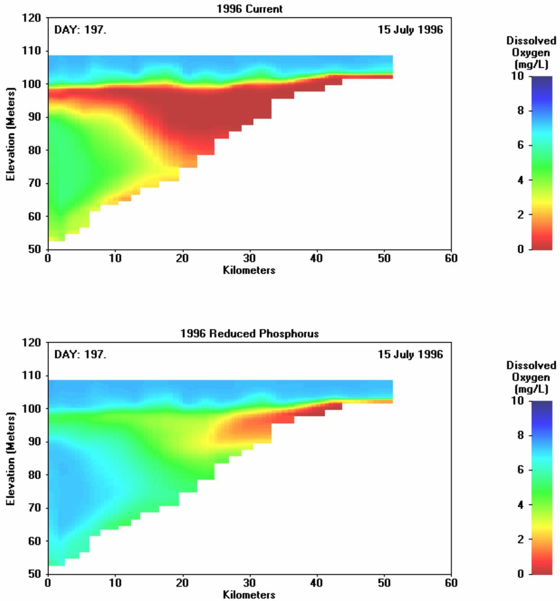
Figure 7-7. 1996 Longitudinal Plots of DO for Current and Reduced Phosphorus on July 15
