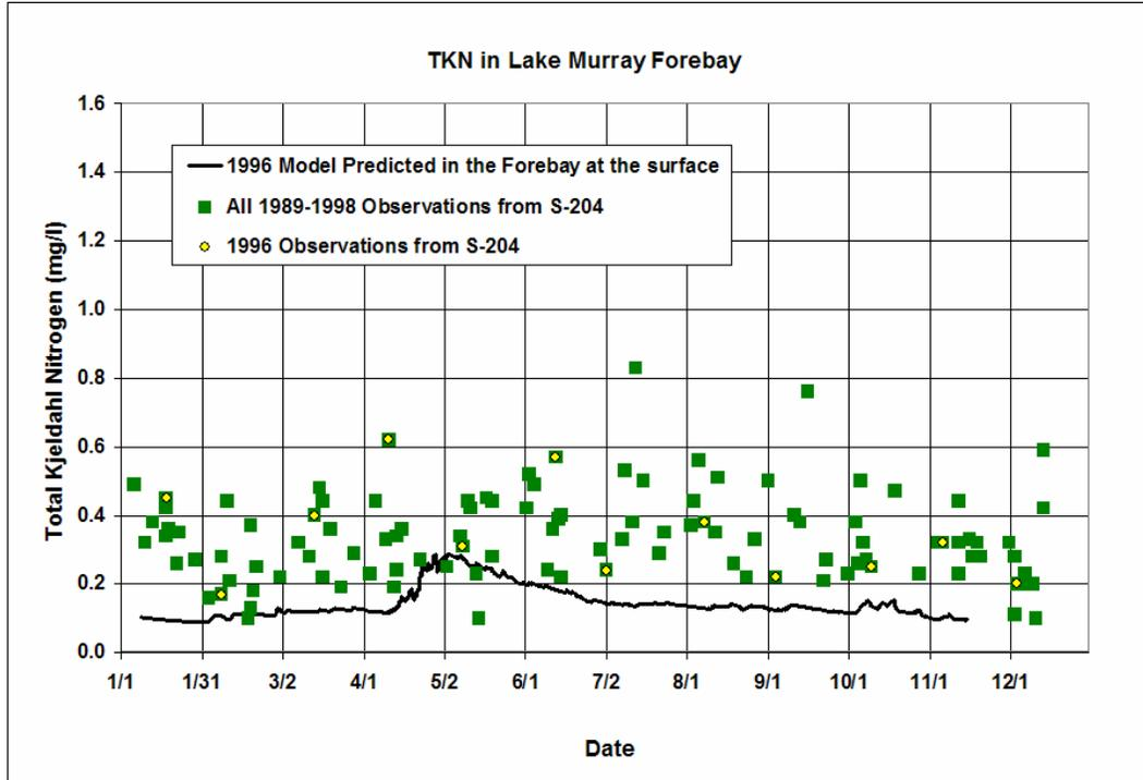
Figure 6-38. 1996 Comparison of Modeled Derived versus Measured TKN at the Surface in the Forebay of Lake Murray
