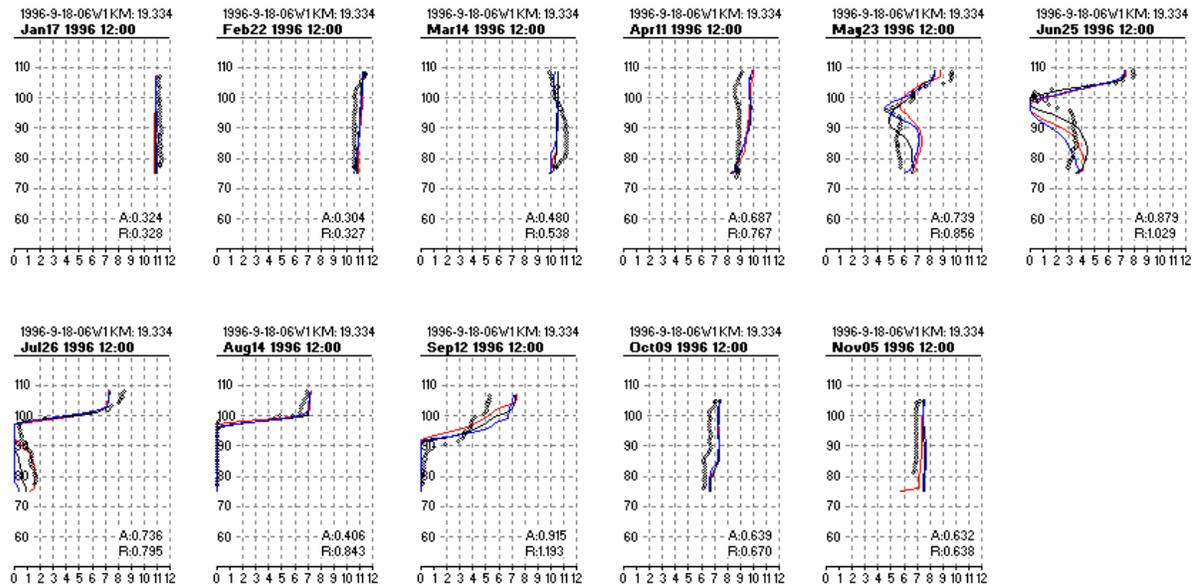
**Figure 6-49. 1996 Modeled and Observed DO Profiles 19 Kilometers Upstream of Saluda Dam; Overall Statistics: ABS = 0.61, RMS = 0.77**
