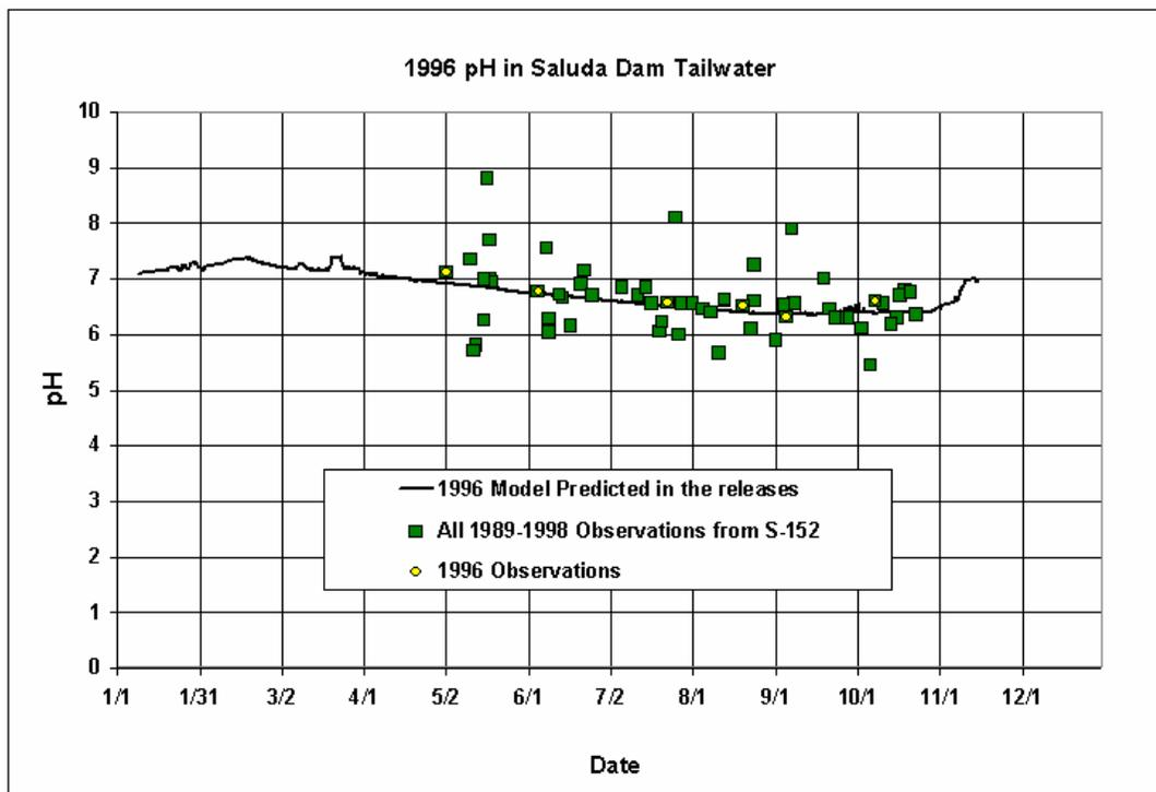
Figure 6-69. 1996 Comparison of Modeled Derived versus Measured pH in the Releases from Saluda Dam
