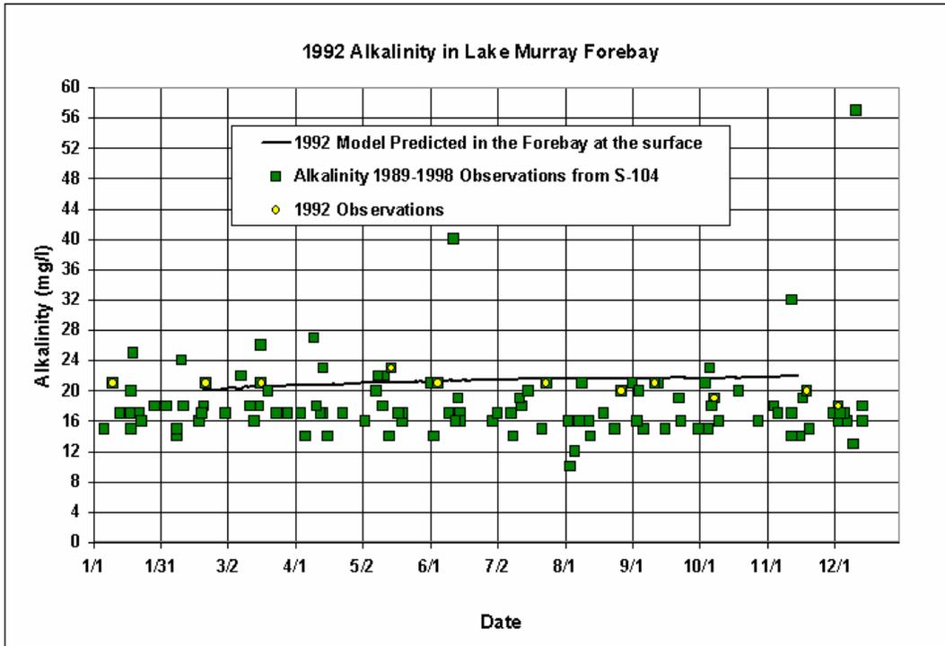
Figure 6-61. 1992 Comparison of Modeled Derived versus Measured Alkalinity at the Surface in the Forebay of Lake Murray
