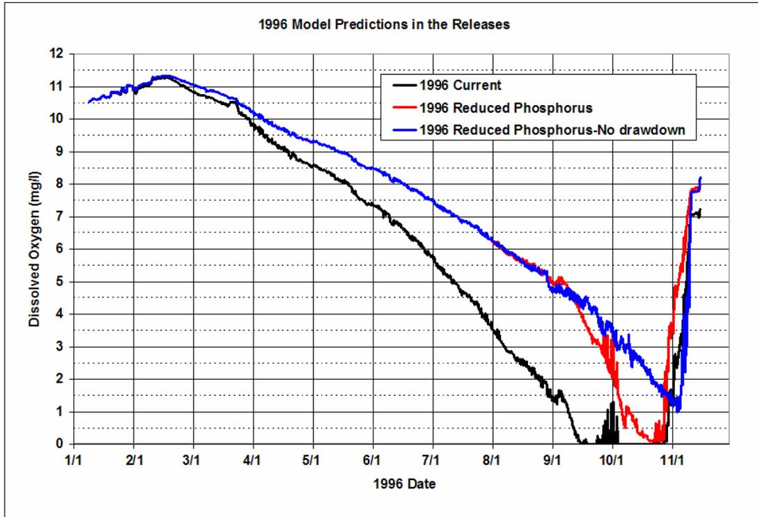
Figure 7-26. 1996 Release DO for Current and Reduced Phosphorus, and without the Special Drawdown
