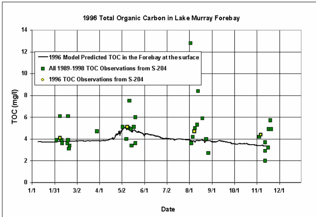
Figure 6-41. 1996 Comparison of Modeled Derived versus Measured TOC at the Surface in the Forebay of Lake Murray
