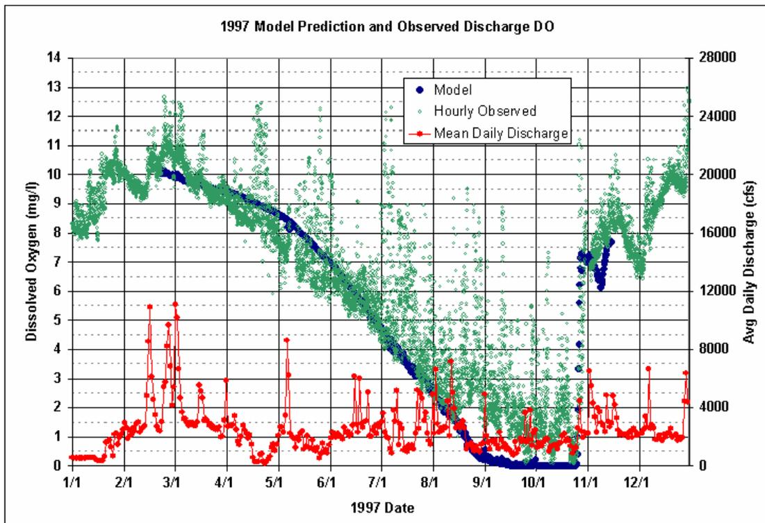
Figure 6-57. 1997 Comparison of Modeled versus Measured Saluda Release DO
