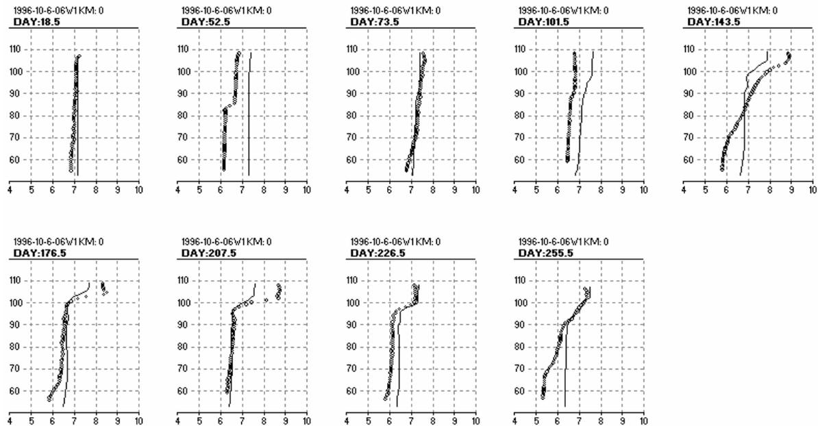
Figure 6-67. 1996 Modeled and Observed pH Profiles in the Forebay of Lake Murray
