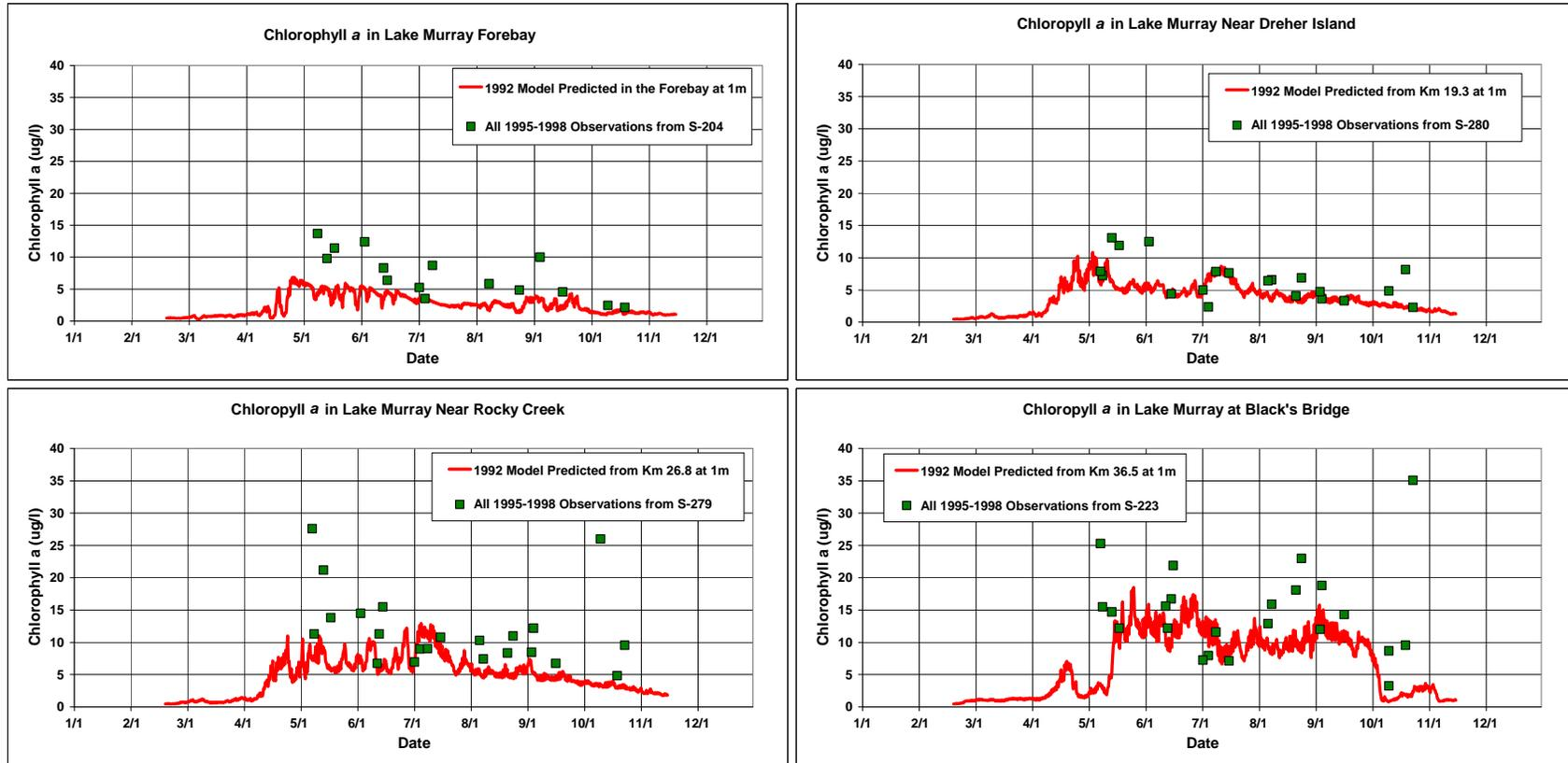
Figure 6-34. 1992 Comparison of Modeled versus Measured Chlorophyll *a* at Four Locations in Lake Murray
