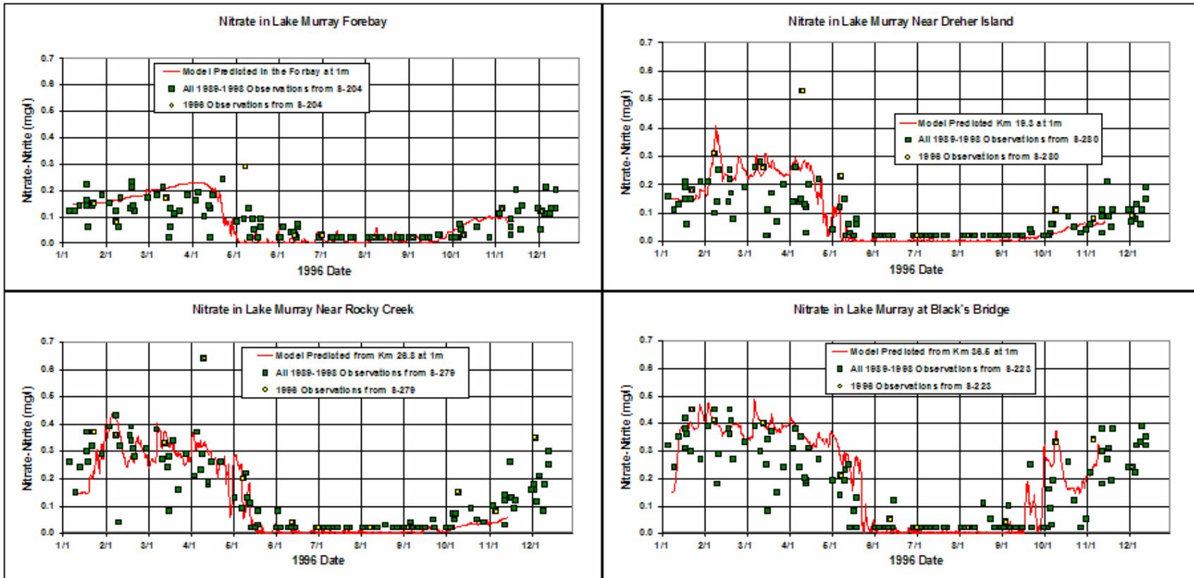
Figure 6-29. 1996 Comparison of Modeled versus Measured Nitrate-Nitrite at Four Locations in Lake Murray
