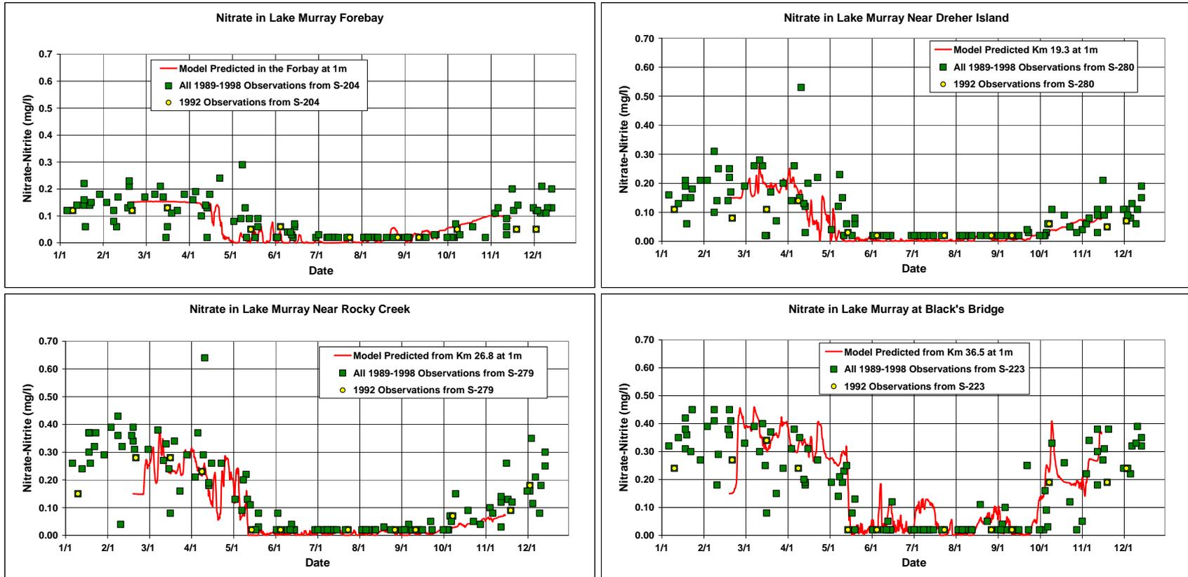
Figure 6-28. 1992 Comparison of Modeled versus Measured Nitrate-Nitrite at Four Locations in Lake Murray
