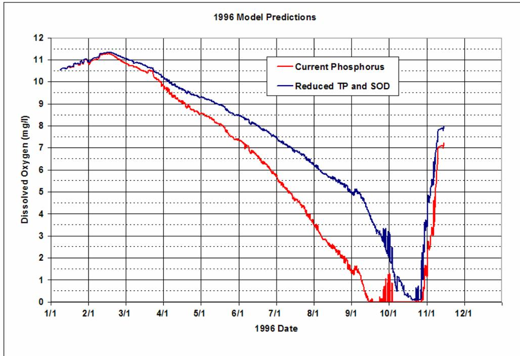
Figure 7-3. 1996 Release DO for Current Phosphorus Loads and Reduced Phosphorus
