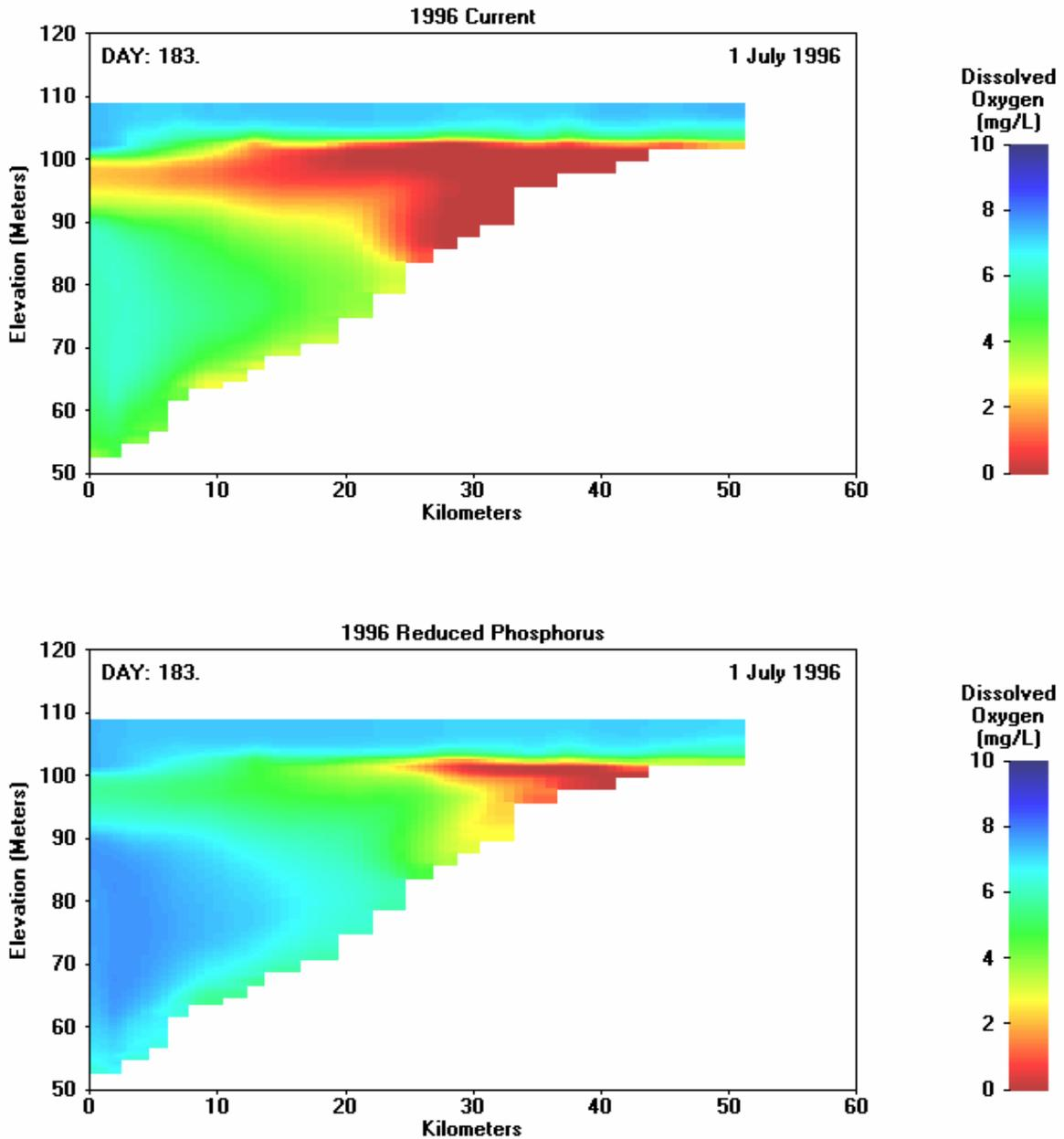
Figure 7-6. 1996 Longitudinal Plots of DO for Current and Reduced Phosphorus on July 1
