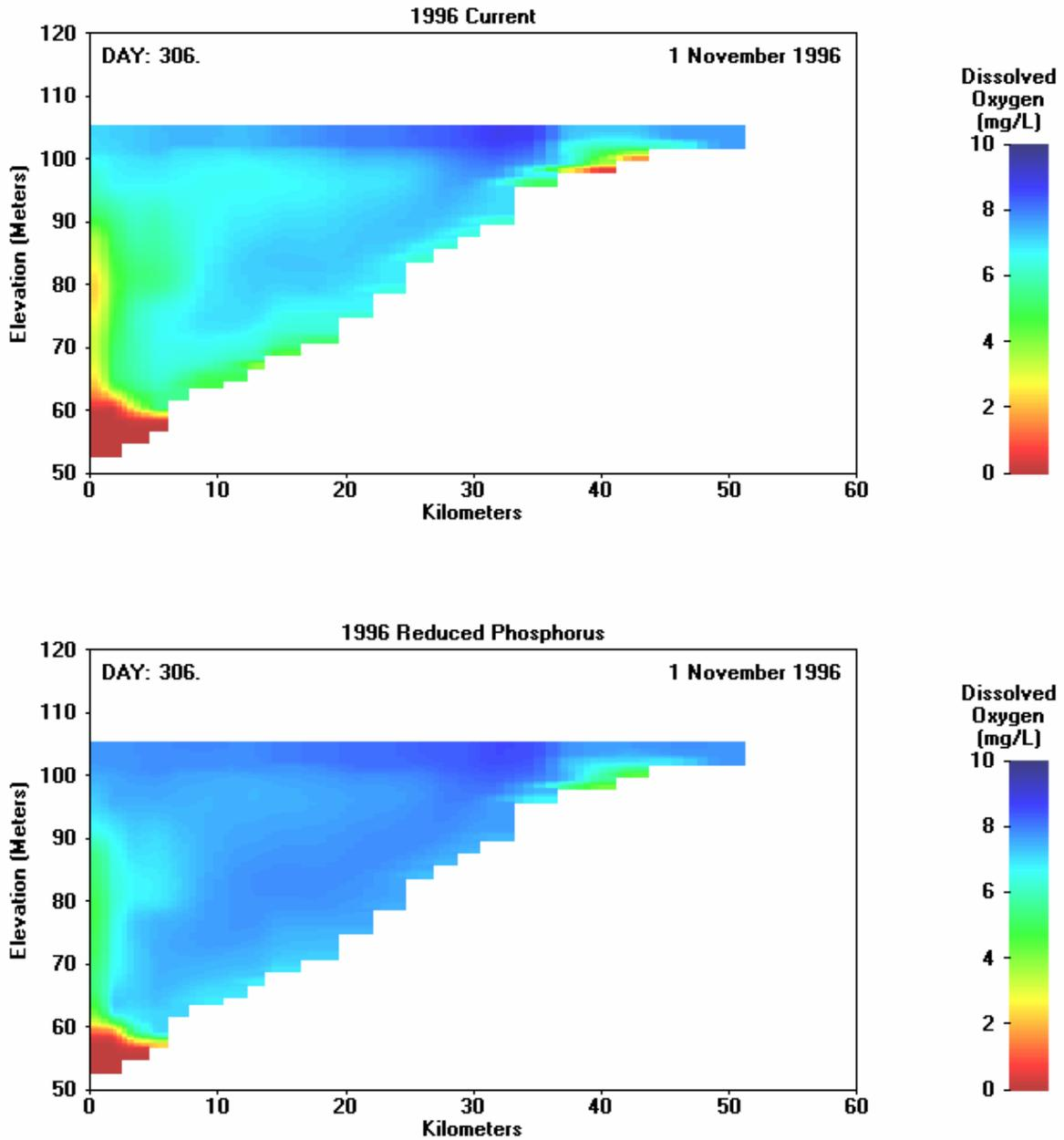
Figure 7-12. 1996 Longitudinal Plots of DO for Current and Reduced Phosphorus on November 1
