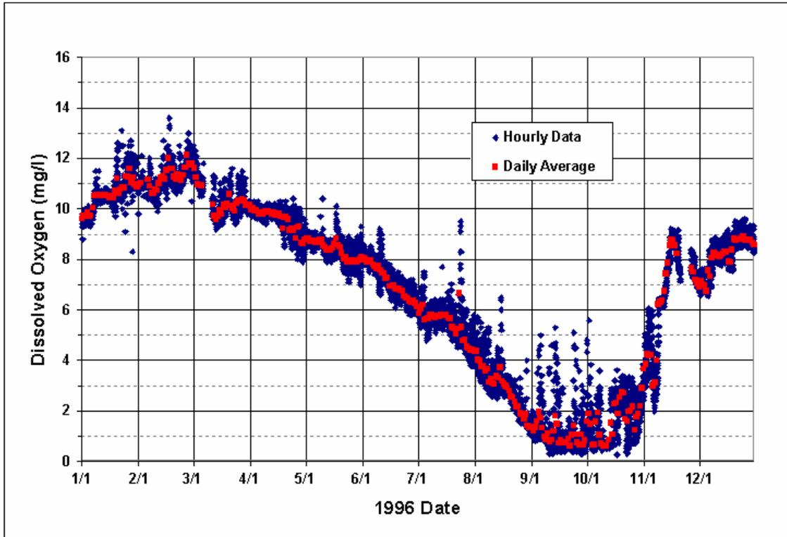
Figure 3-20. DO Measured by USGS in the Saluda Hydro Tailrace in 1996
