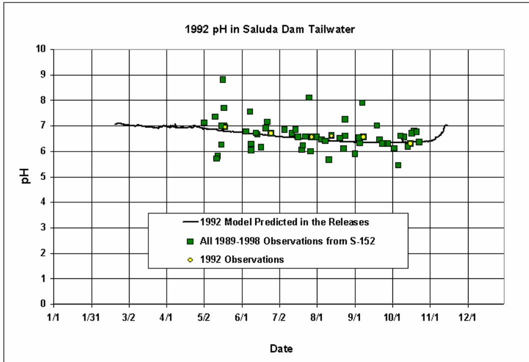
Figure 6-68. 1992 Comparison of Modeled Derived versus Measured pH in the Releases from Saluda Dam
