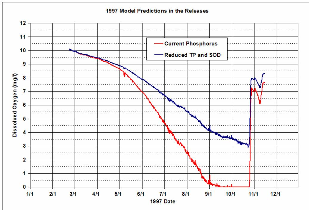
Figure 7-4. 1997 Release DO for Current Phosphorus Loads and Reduced Phosphorus
