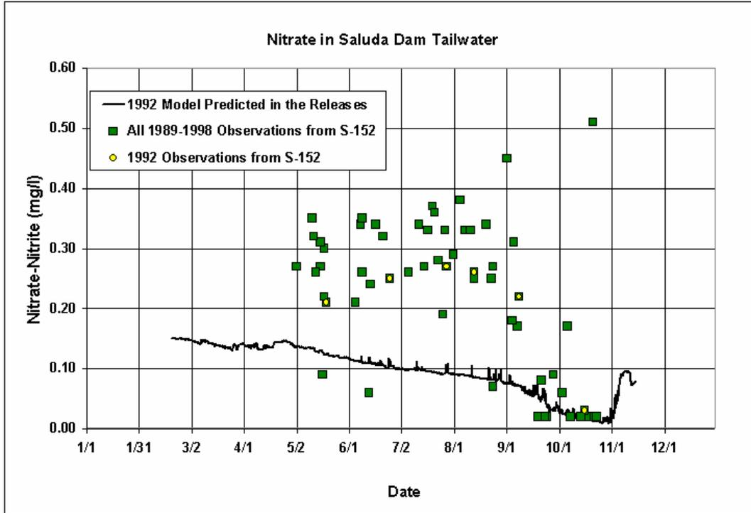
Figure 6-31. 1992 Comparison of Modeled Derived versus Measured Nitrate in the Releases from Saluda Dam
