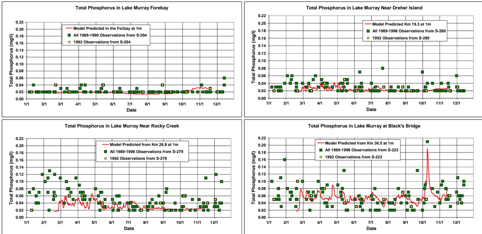
Figure 6-22. 1992 Comparison of Modeled Derived versus Measured Total Phosphorus at Four Locations in Lake Murray
