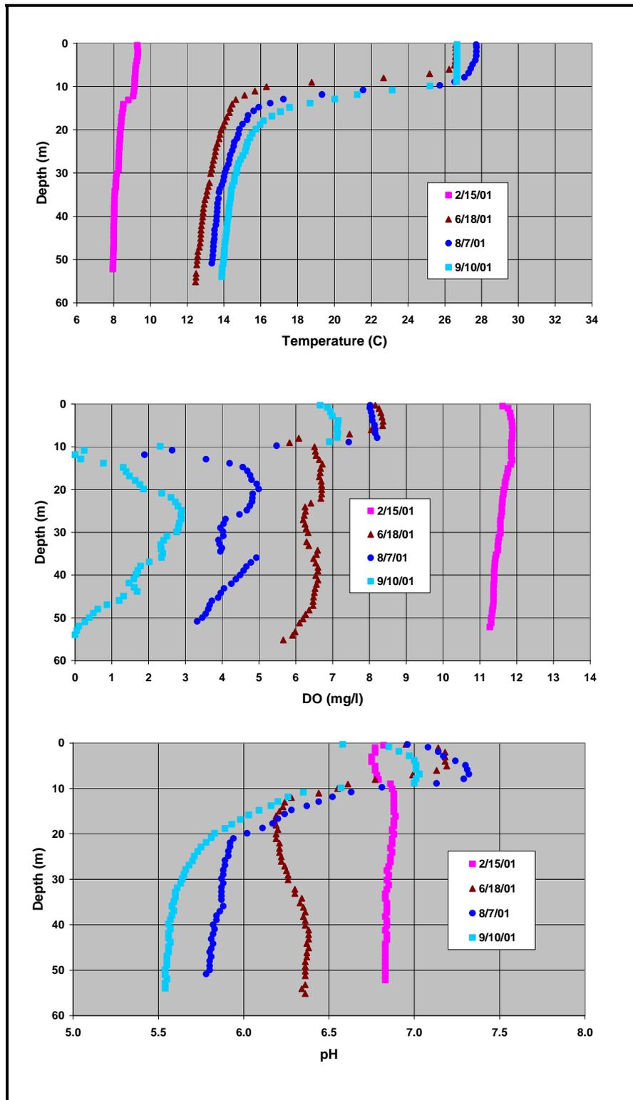
**Figure 3-19. Temperature, DO, and pH profiles from 2001 showing the correlation between pH and low DO**
