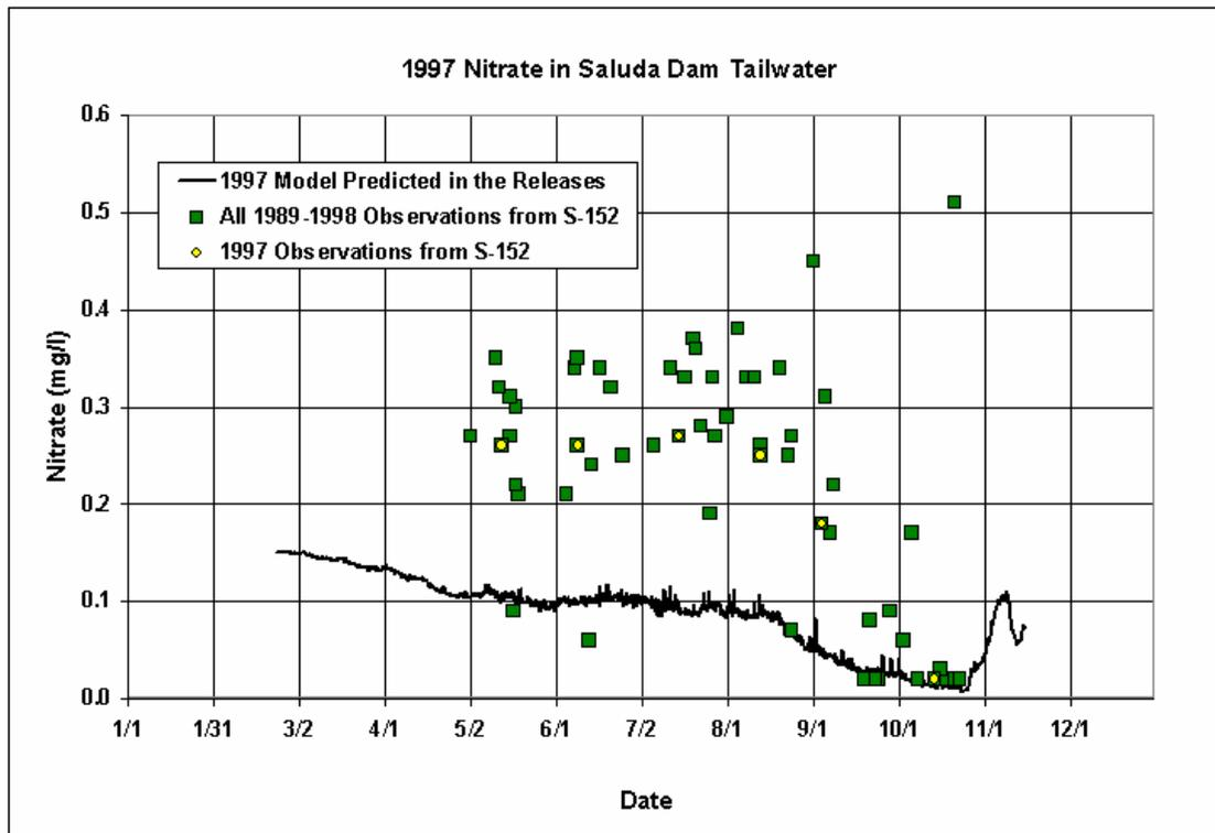
**Figure 6-33. 1997 Comparison of Modeled Derived versus Measured Nitrate in the Releases from Saluda Dam**
