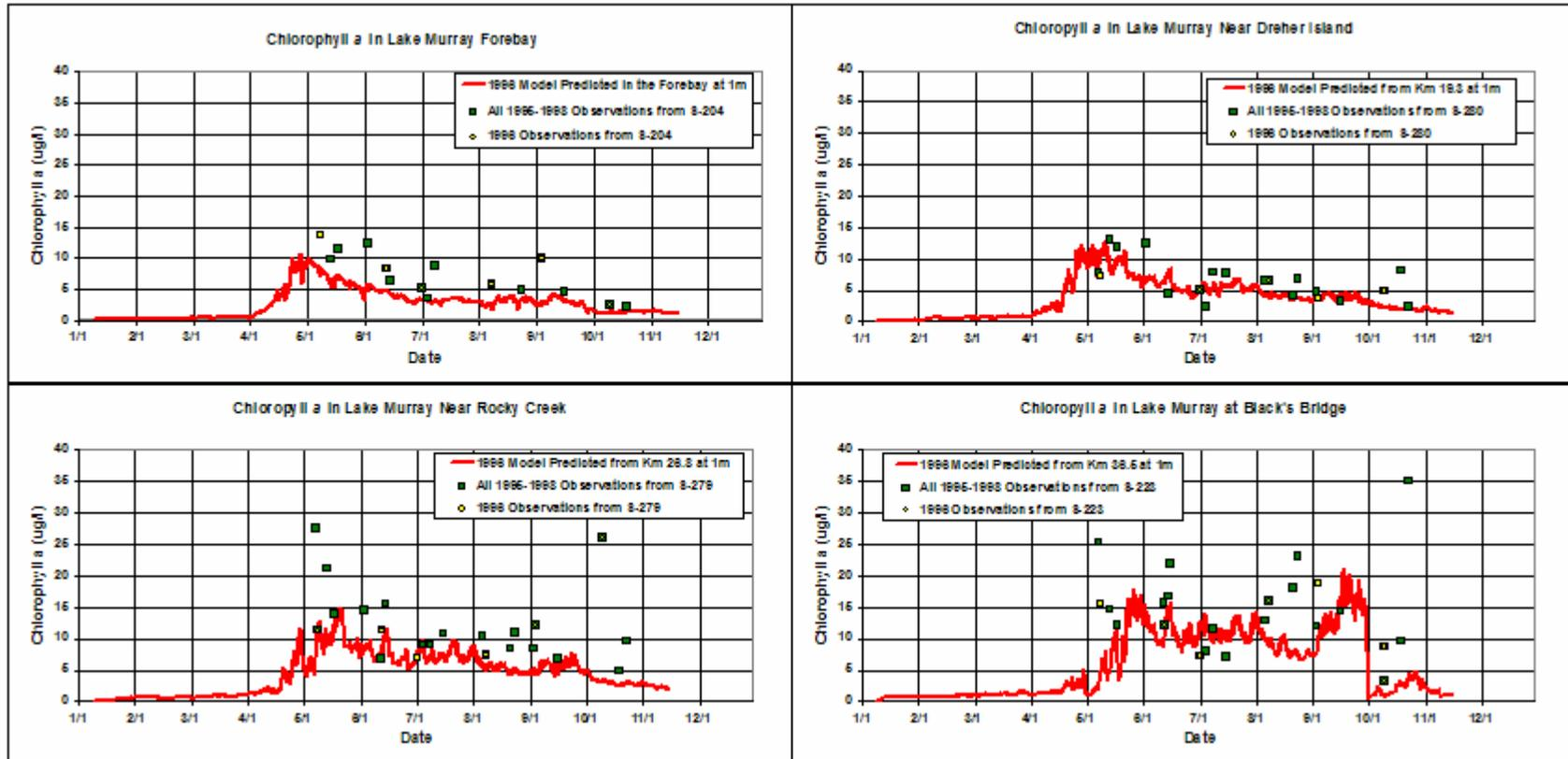
Figure 6-35. 1996 Comparison of Modeled versus Measured Chlorophyll *a* at Four Locations in Lake Murray
