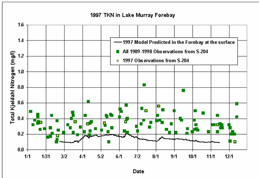
Figure 6-39. 1997 Comparison of Modeled Derived versus Measured TKN at the Surface in the Forebay of Lake Murray
