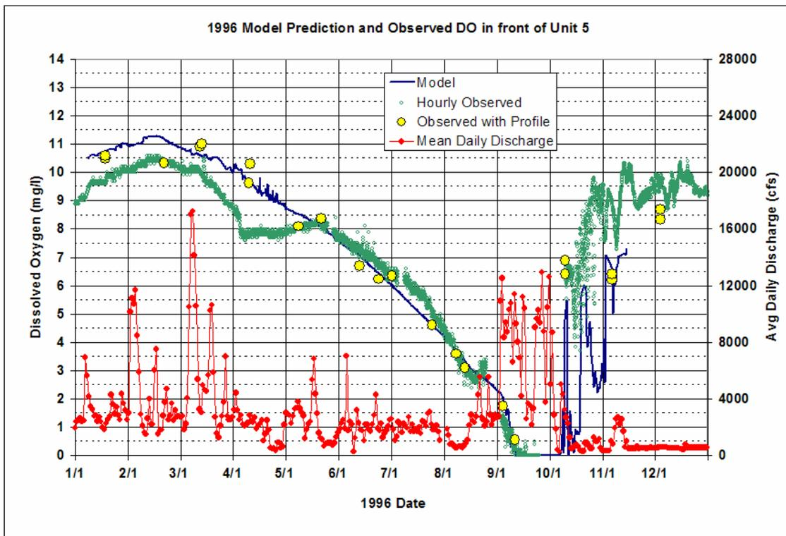
Figure 6-59. 1996 Modeled versus Measured DO at the level of the Unit 5 Intake
