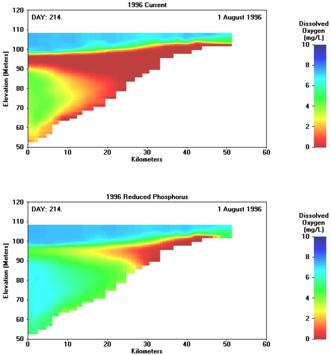
Figure 7-8. 1996 Longitudinal Plots of DO for Current and Reduced Phosphorus Day on August 1
