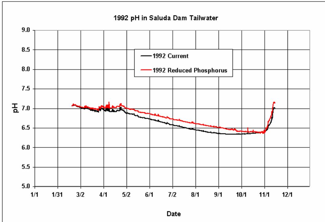
**Figure 7-22. Comparison of 1992 Current and Reduced Phosphorus Predictions of pH in the Releases from Saluda Hydro**
