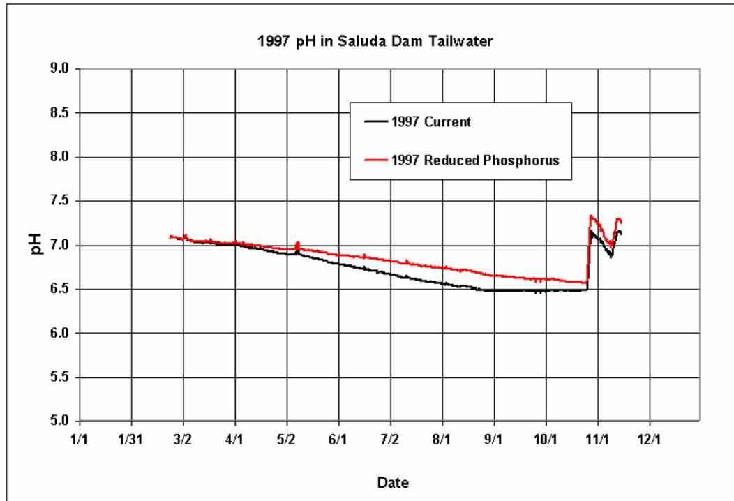
**Figure 7-24. Comparison of 1997 Current and Reduced Phosphorus Predictions of pH in the Releases from Saluda Hydro**
