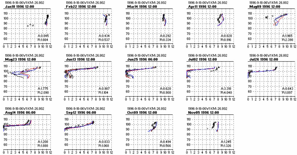
**Figure 6-50. 1996 Modeled and Observed DO Profiles 27 Kilometers Upstream of Saluda Dam; Overall Statistics: ABS = 1.01, RMS = 1.54**
