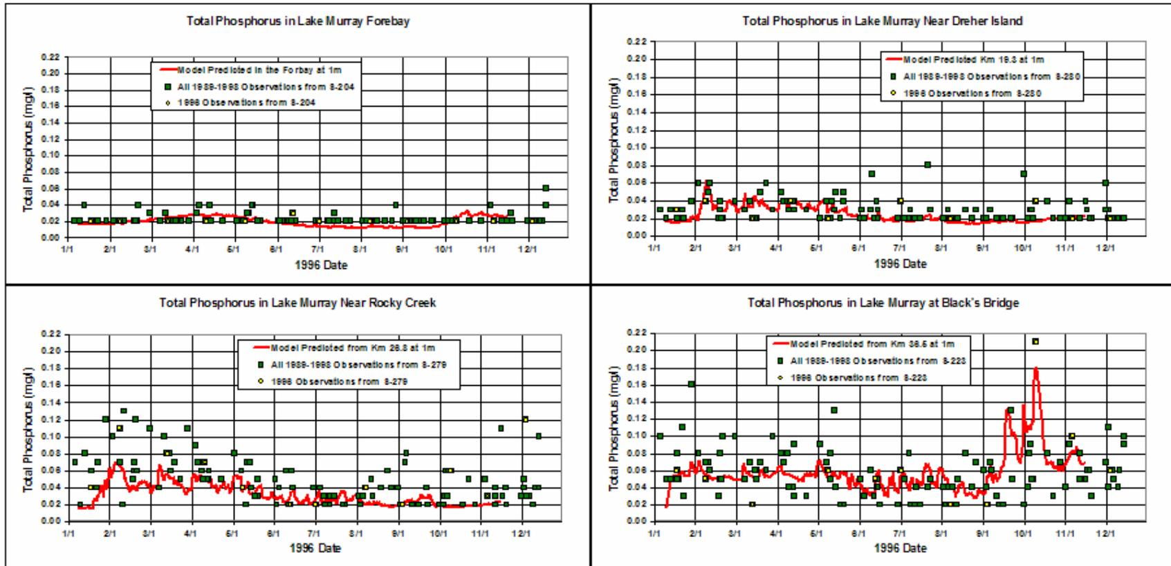
Figure 6-23. 1996 Comparison of Modeled Derived versus Measured Total Phosphorus at Four Locations in Lake Murray
