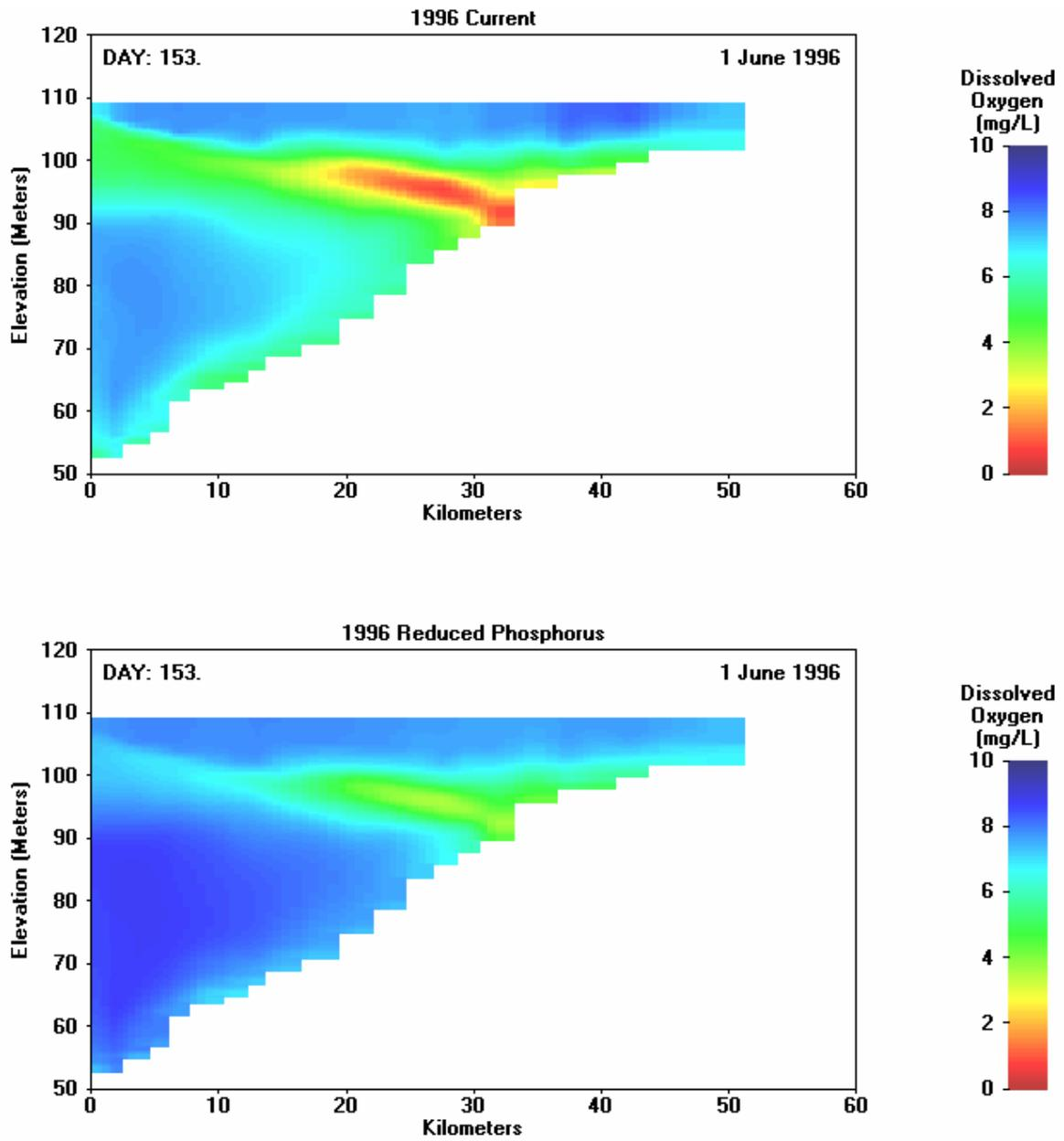
Figure 7-5. 1996 Longitudinal Plots of DO for Current and Reduced Phosphorus on June 1
