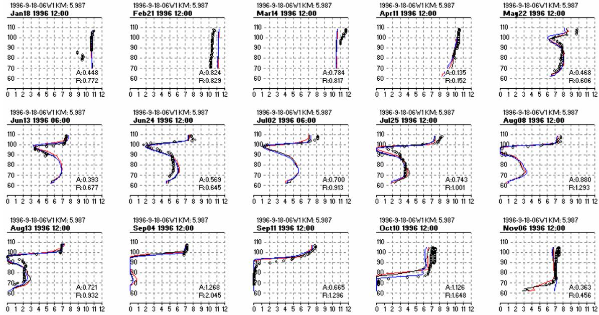
**Figure 6-48. 1996 Modeled and Observed DO Profiles Six Kilometers Upstream of Saluda Dam; Overall Statistics: ABS = 0.65, RMS = 1.00**
