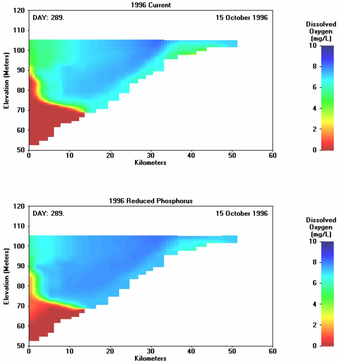
Figure 7-11. 1996 Longitudinal Plots of DO for Current and Reduced Phosphorus on October 15
