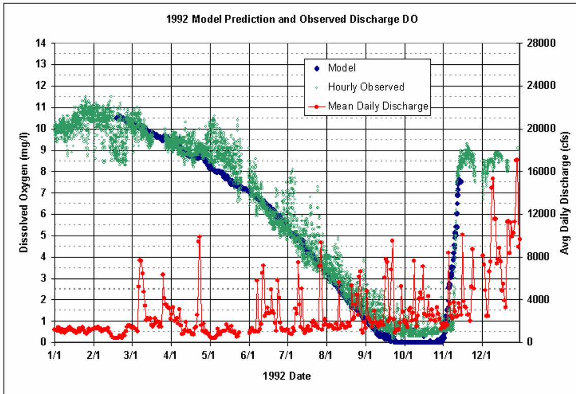
Figure 6-55. 1992 Comparison of Modeled versus Measured Saluda Release DO
