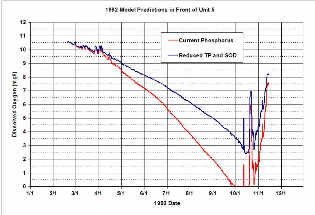
Figure 7-16. 1992 DO at the Level of the Unit 5 Intake for Current and Reduced Phosphorus
