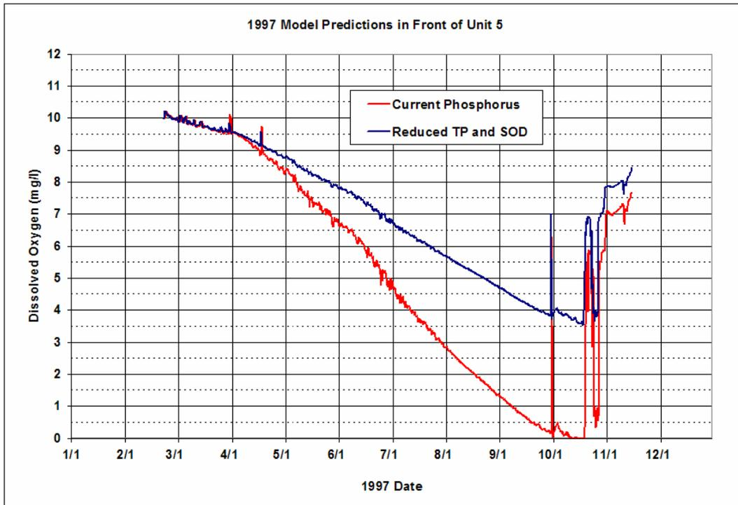
**Figure 7-18. 1997 DO at the Level of the Unit 5 Intake for Current and Reduced Phosphorus**
