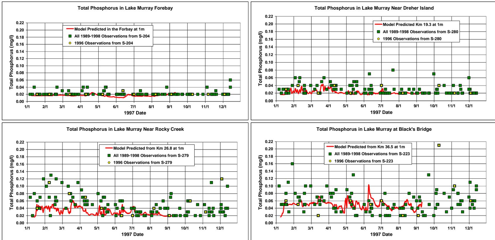
Figure 6-24. 1997 Comparison of Modeled Derived versus Measured Total Phosphorus at Four Locations in Lake Murray
