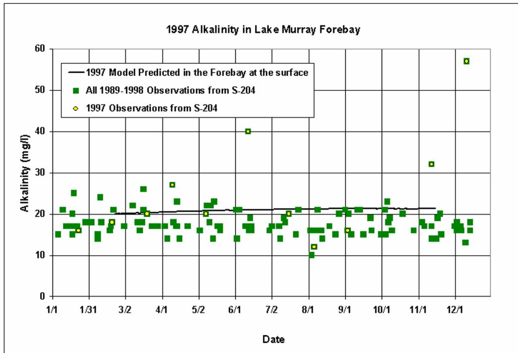
Figure 6-63. 1997 Comparison of Modeled Derived versus Measured Alkalinity at the Surface in the Forebay of Lake Murray
