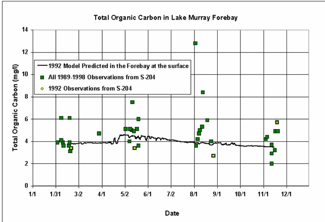
Figure 6-40. 1992 Comparison of Modeled Derived versus Measured TOC at the Surface in the Forebay of Lake Murray
