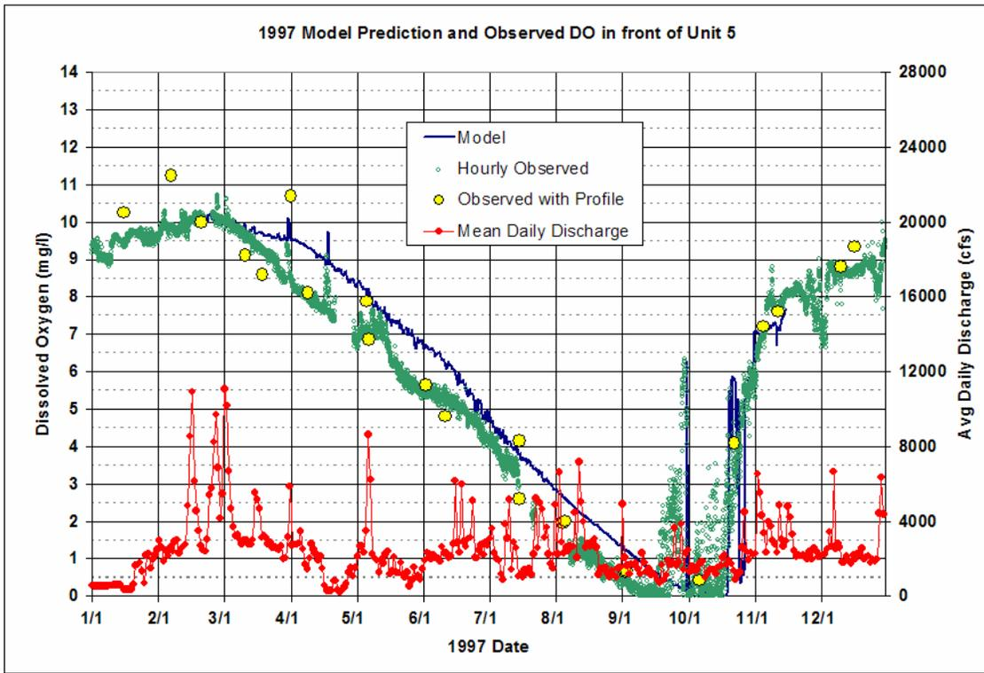
Figure 6-60. 1997 Modeled versus Measured DO at the level of the Unit 5 Intake
