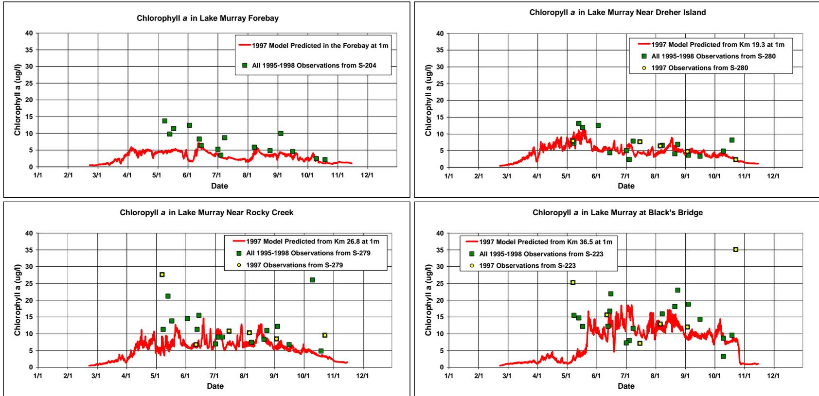
Figure 6-36. 1997 Comparison of Modeled versus Measured Chlorophyll *a* at Four Locations in Lake Murray
