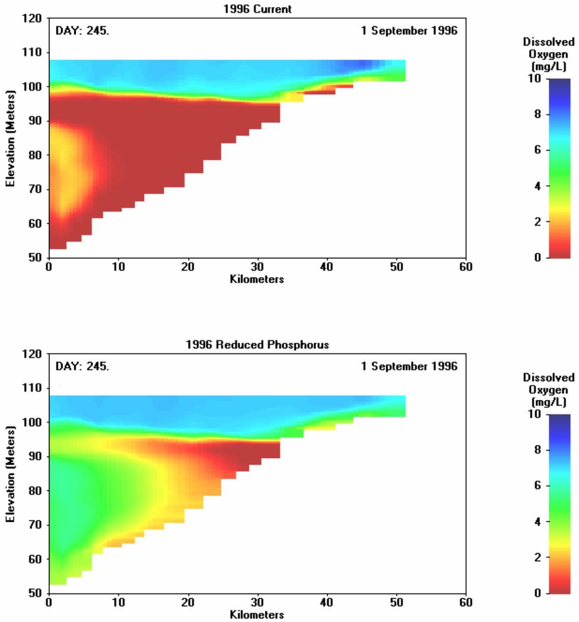
Figure 7-9. 1996 Longitudinal Plots of DO for Current and Reduced Phosphorus on September 1
