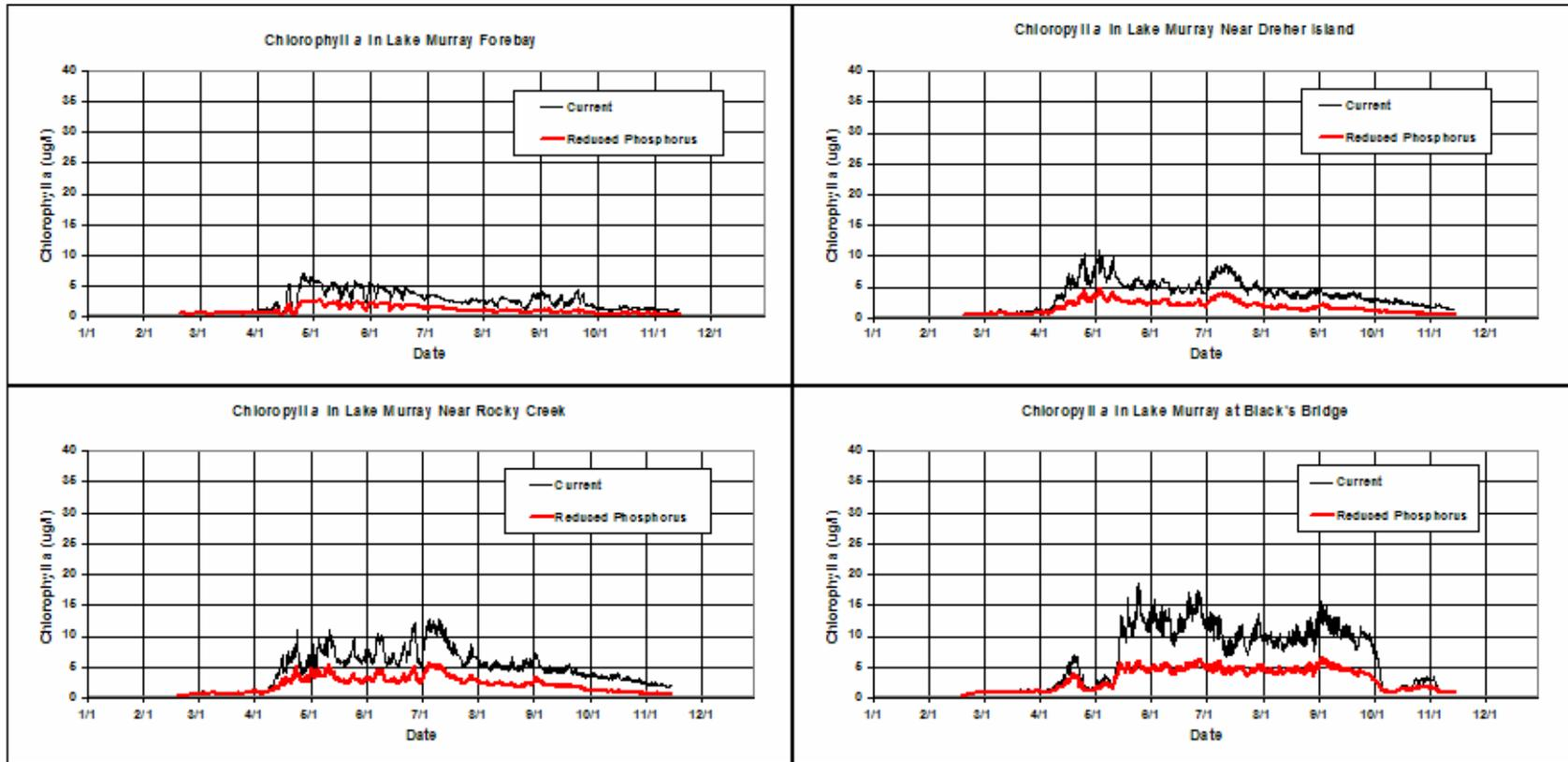
Figure 7-19. Comparison of 1992 Current and Reduced Phosphorus Predictions of Chlorophyll *a* at 1 Meter Depth at Four Locations in Lake Murray
