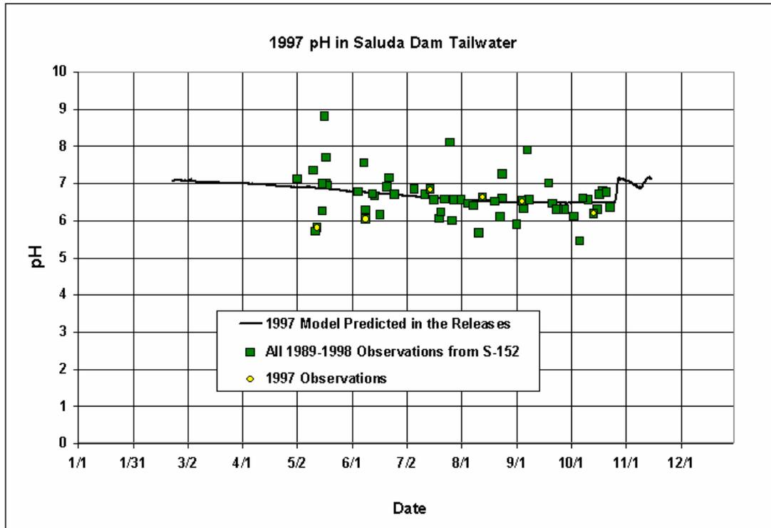
Figure 6-70. 1997 Comparison of Modeled Derived versus Measured pH in the Releases from Saluda Dam
