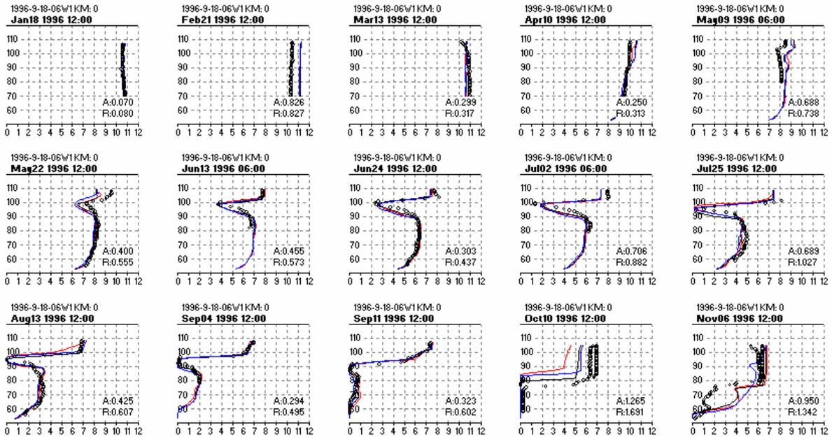
Figure 6-47. 1996 Modeled and Observed DO Profiles in the Forebay of Lake Murray; Overall Statistics: ABS = 0.57, RMS = 0.89
