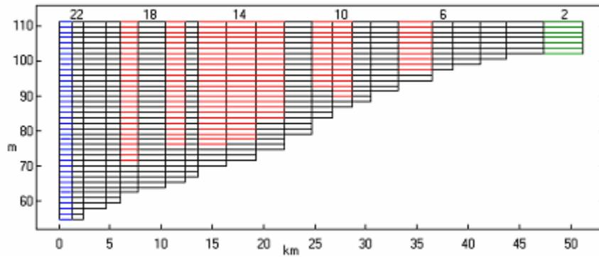
**Figure 5-5. Side View of CE-QUAL-W2 Bathymetry for the Main Branch (Branch 1) of Lake Murray**
