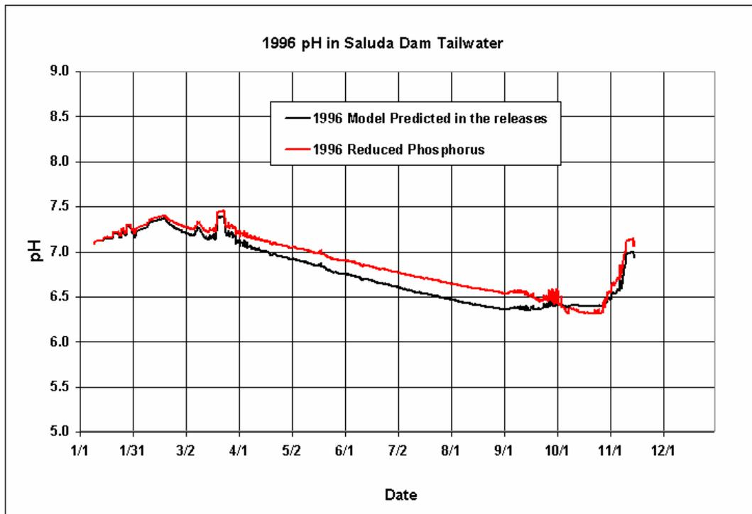
**Figure 7-23. Comparison of 1996 Current and Reduced Phosphorus Predictions of pH in the Releases from Saluda Hydro**
