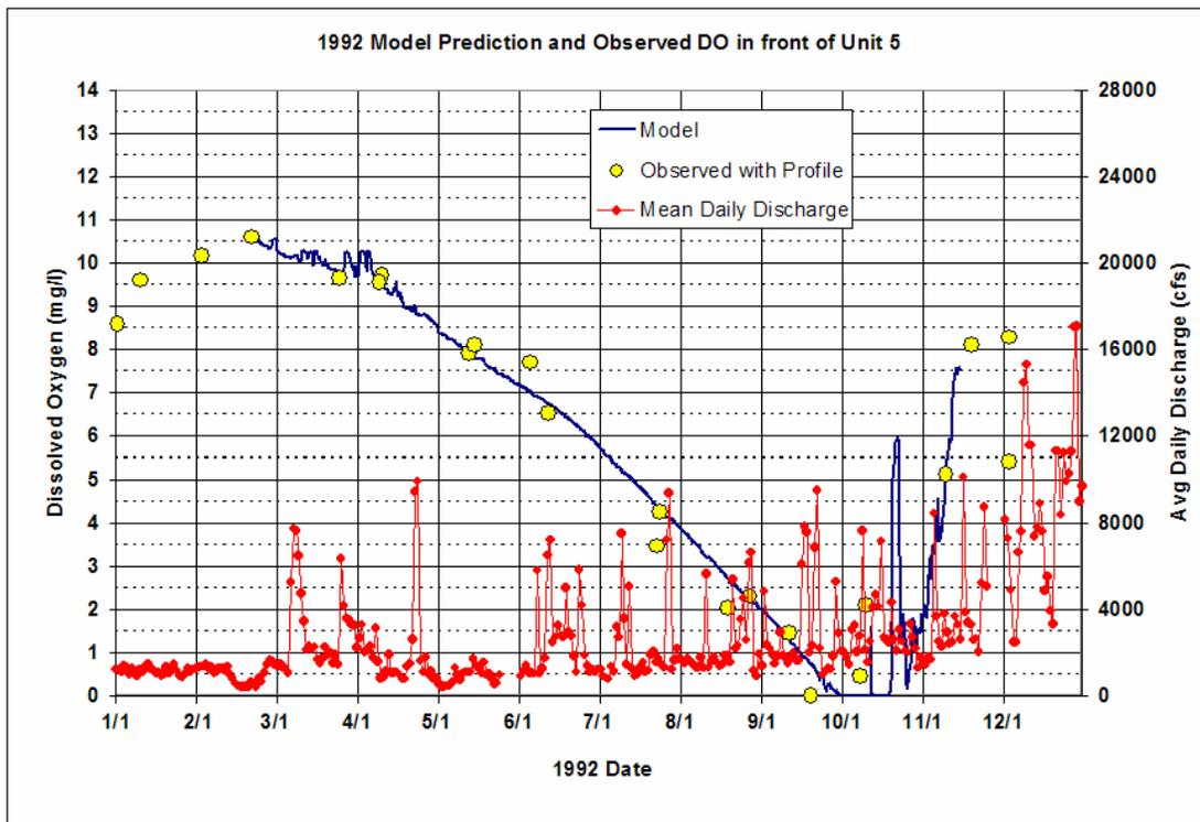
Figure 6-58. 1992 Modeled versus Measured DO at the level of the Unit 5 Intake
