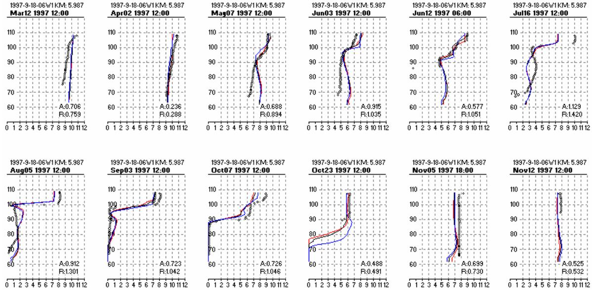
**Figure 6-52. 1997 Modeled and Observed DO Profiles Six Kilometers Upstream of Saluda Dam; Overall Statistics: ABS = 0.72, RMS = 0.98**
