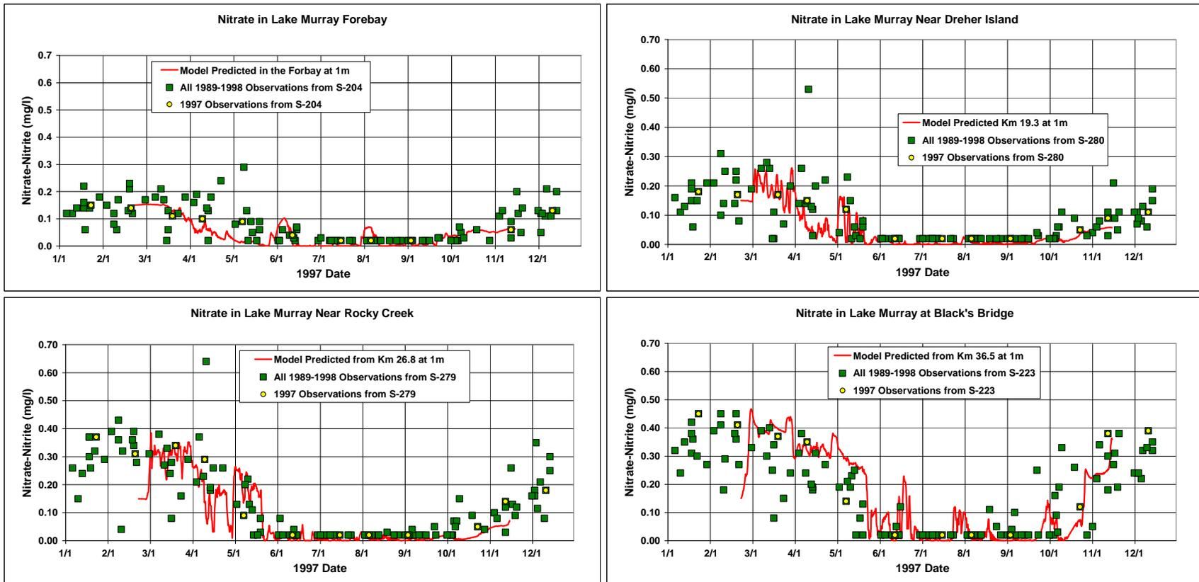
Figure 6-30. 1997 Comparison of Modeled versus Measured Nitrate-Nitrite at Four Locations in Lake Murray
