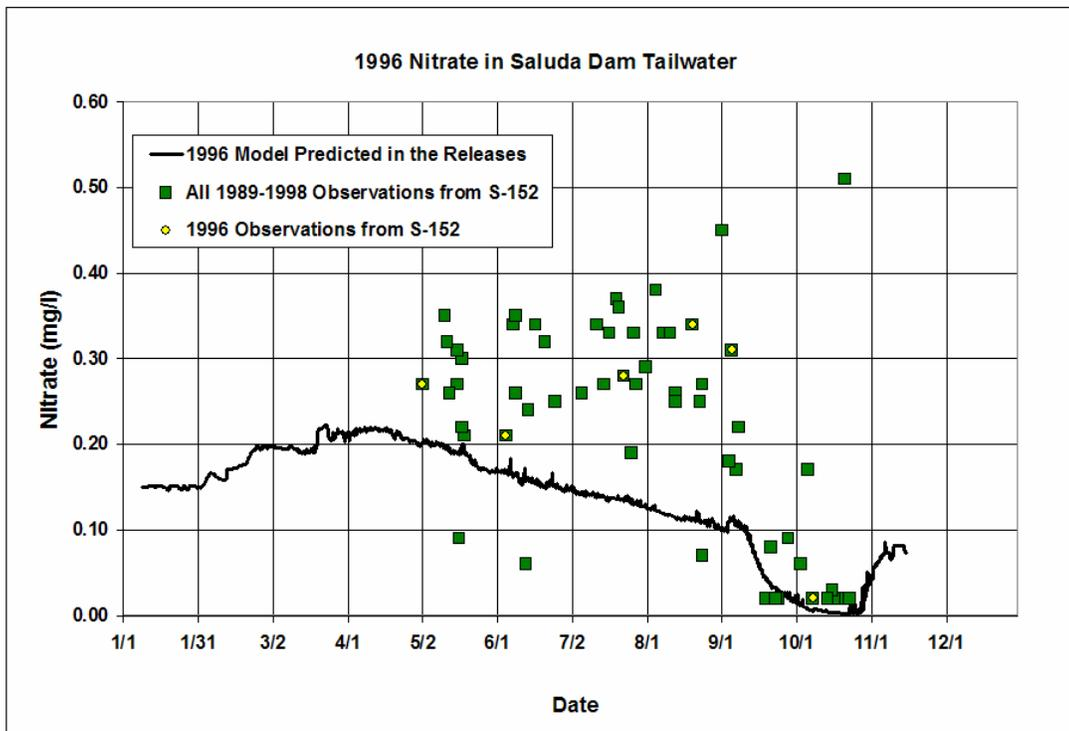
Figure 6-32. 1996 Comparison of Modeled Derived versus Measured Nitrate in the Releases from Saluda Dam
