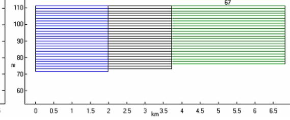
Figure 5-6. Side View of CE-QUAL-W2 Bathymetry for Lake Murray Branches 2-9
