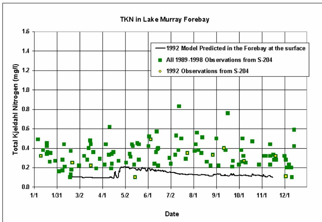
**Figure 6-37. 1992 Comparison of Modeled Derived versus Measured TKN at the Surface in the Forebay of Lake Murray**
