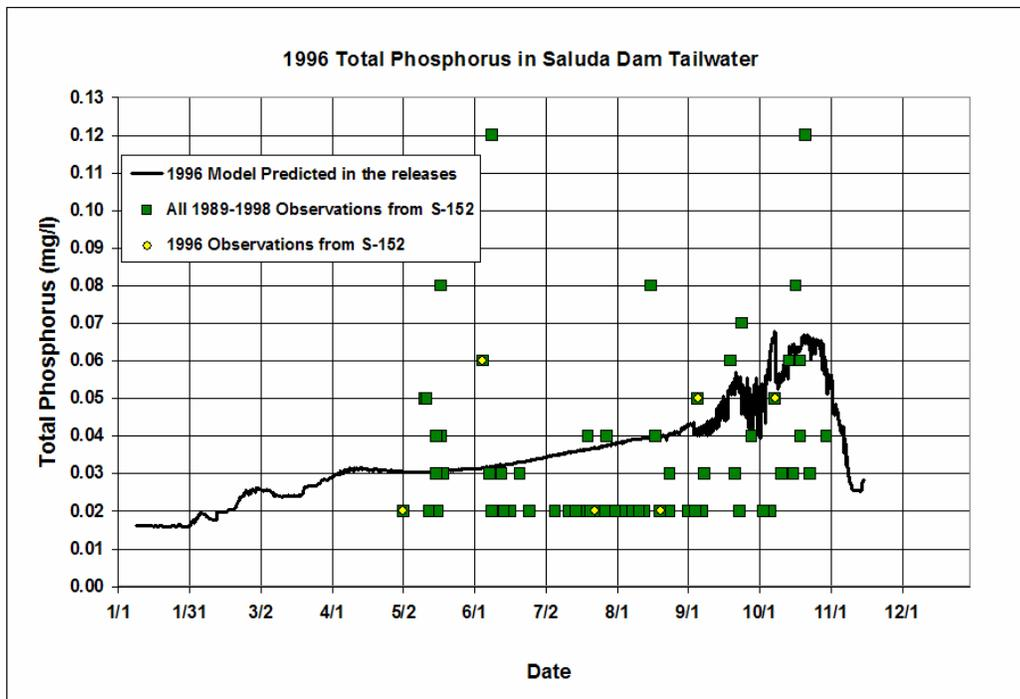
**Figure 6-26. 1996 Comparison of Modeled Derived versus Measured Total Phosphorus in the Releases from Saluda Dam**
