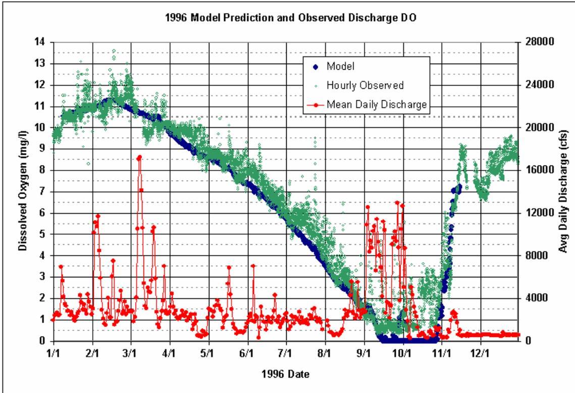
Figure 6-56. 1996 Comparison of Modeled versus Measured Saluda Release DO
