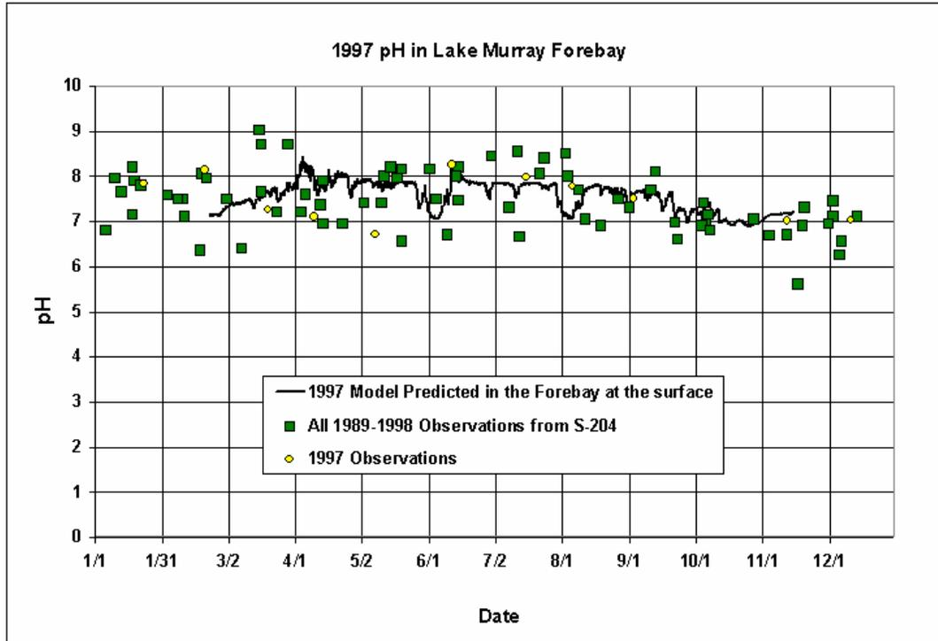
Figure 6-66. 1997 Comparison of Modeled Derived versus Measured pH at the Surface in the Forebay of Lake Murray
