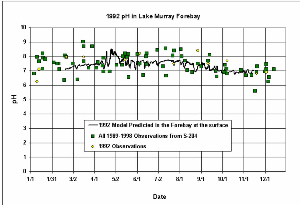
**Figure 6-64. 1992 Comparison of Modeled Derived versus Measured pH at the Surface in the Forebay of Lake Murray**
