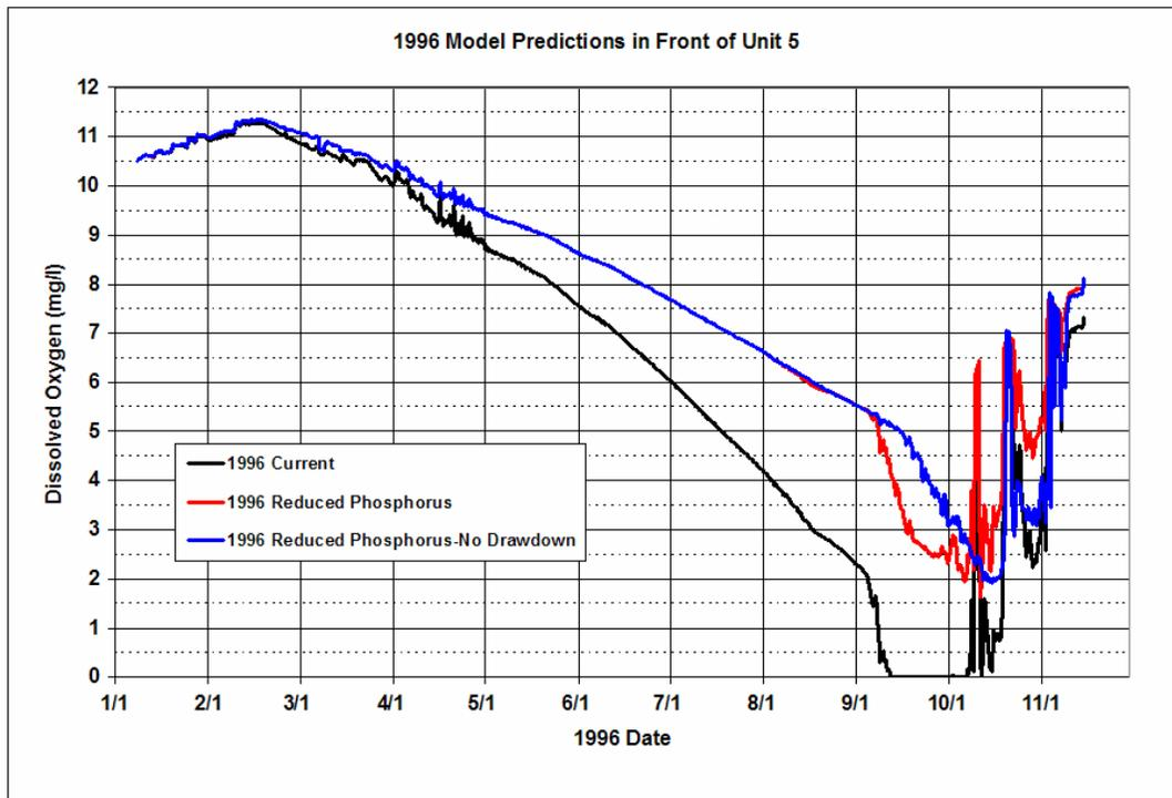
Figure 7-27. 1996 DO at the Elevation of the Unit 5 Intake for Current and Reduced Phosphorus, and without the Special Drawdown
