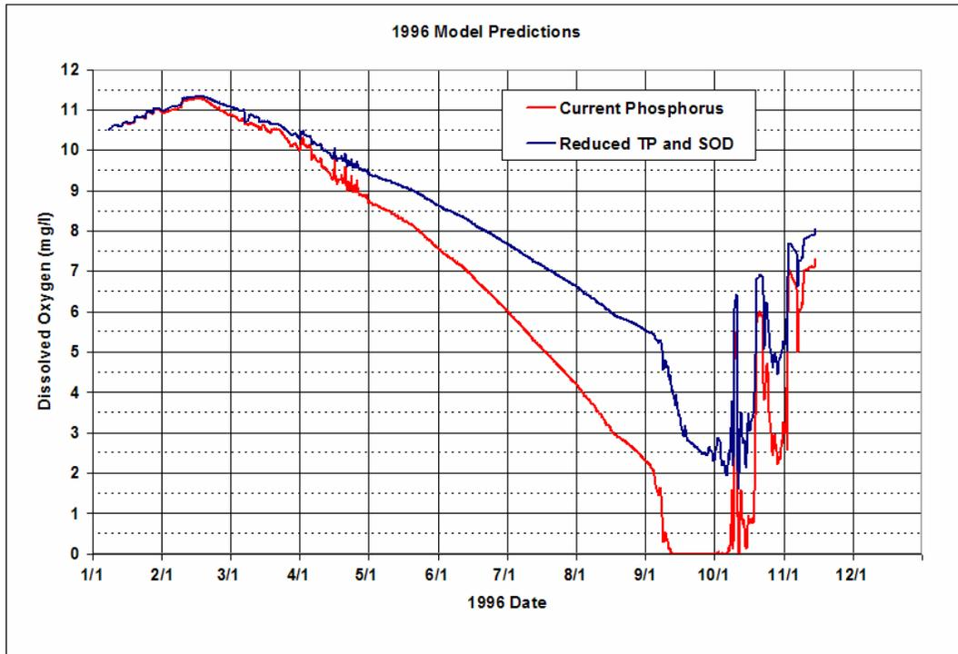
Figure 7-17. 1996 DO at the Level of the Unit 5 Intake for Current and Reduced Phosphorus
