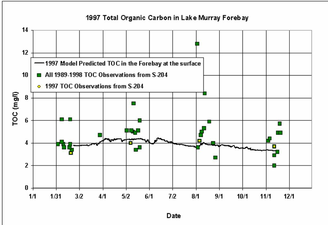
Figure 6-42. 1997 Comparison of Modeled Derived versus Measured TOC at the Surface in the Forebay of Lake Murray
