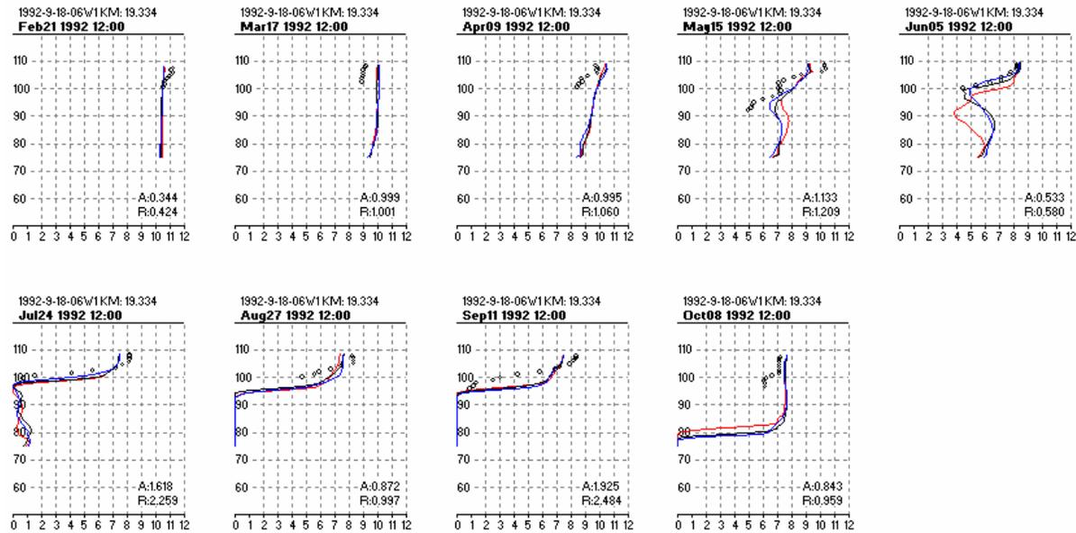
**Figure 6-45. 1992 Modeled and Observed DO Profiles 19 Kilometers Upstream of Saluda Dam; Overall Statistics: ABS = 1.08, RMS = 1.44**
