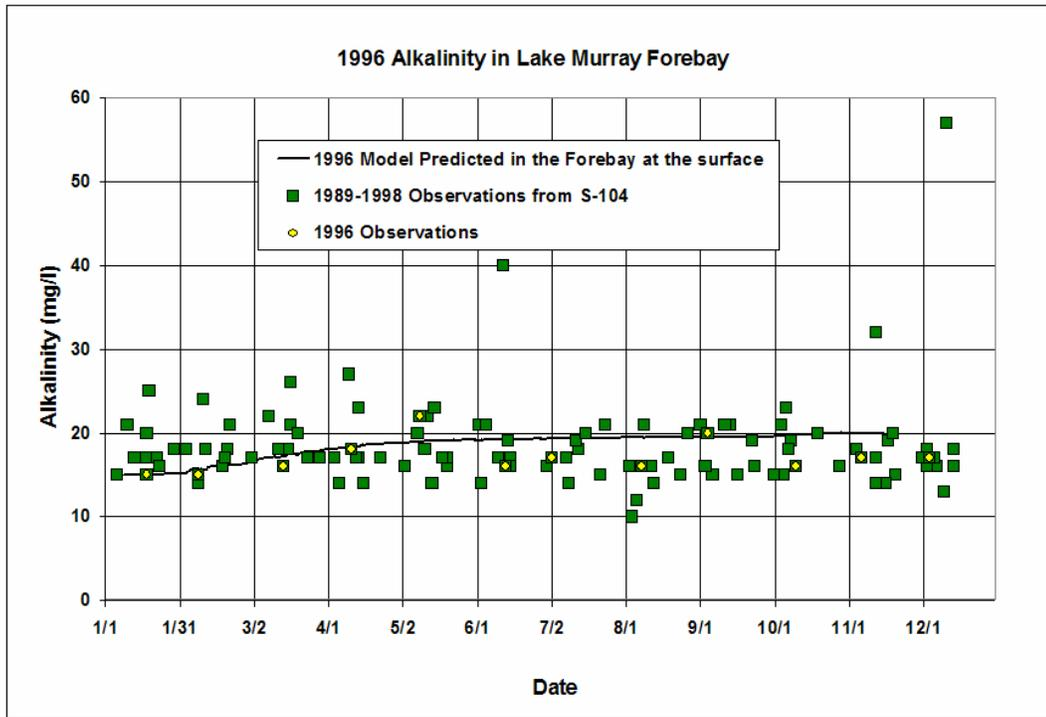
Figure 6-62. 1996 Comparison of Modeled Derived versus Measured Alkalinity at the Surface in the Forebay of Lake Murray
