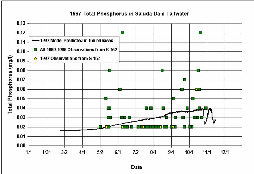
Figure 6-27. 1997 Comparison of Modeled Derived versus Measured Total Phosphorus in the Releases from Saluda Dam
