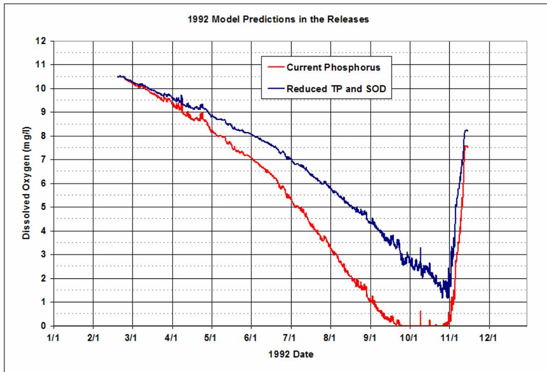
**Figure 7-2. 1992 Release DO for Current Phosphorus Loads and Reduced Phosphorus**
