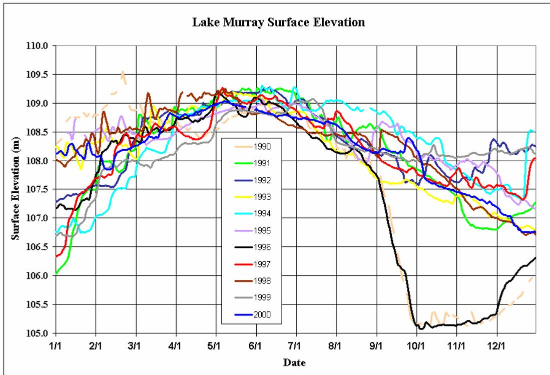
**Figure 7-25. Water Surface Elevations for Various Years at Lake Murray**
