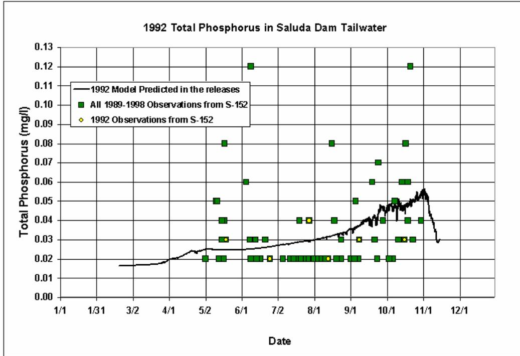
**Figure 6-25. 1992 Comparison of Modeled Derived versus Measured Total Phosphorus in the Releases from Saluda Dam**
