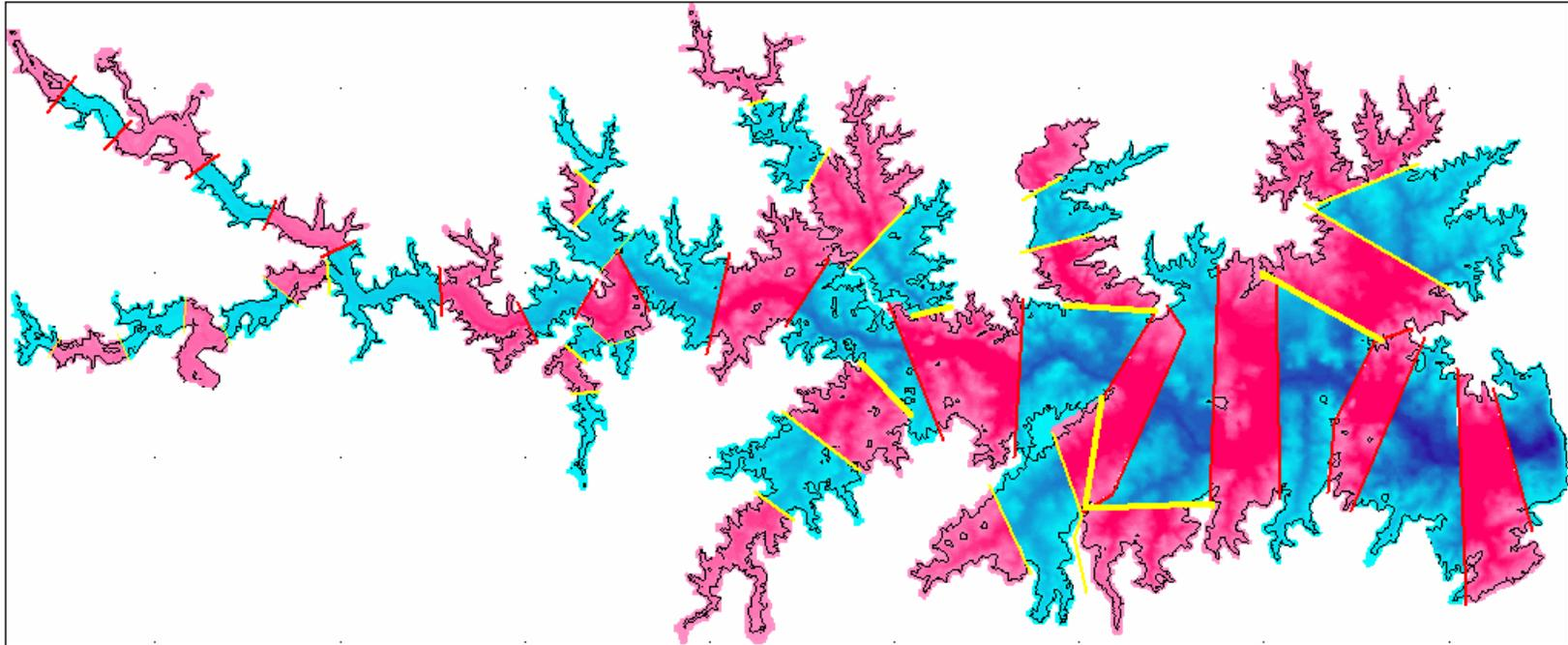
Figure 5-2. Plan View of Lake Murray Showing CE-QUAL-W2 Segmentation
