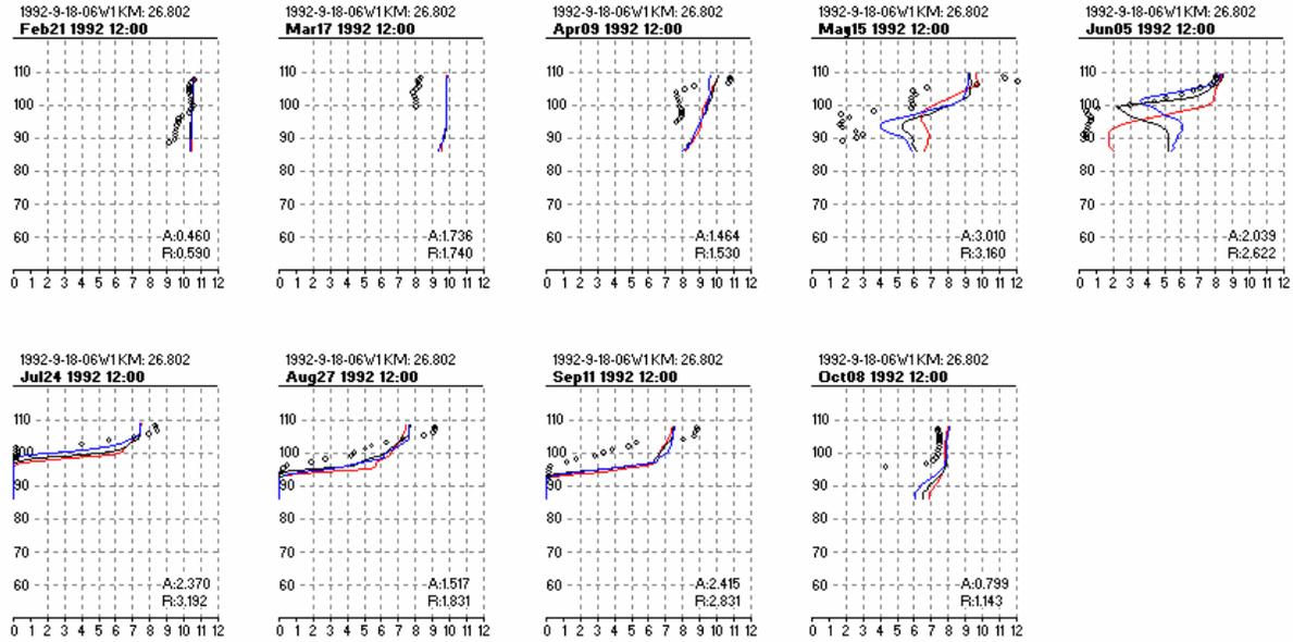
Figure 6-46. 1992 Modeled and Observed DO Profiles 27 Kilometers Upstream of Saluda Dam; Overall Statistics: ABS = 1.78, RMS = 2.28
