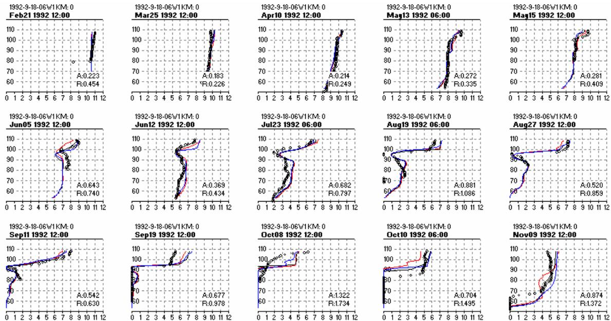
Figure 6-43. 1992 Modeled and Observed DO Profiles in the Forebay of Lake Murray; Overall Statistics: ABS = 0.55, RMS = 0.90
