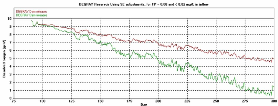
**Figure 3-22. CE-QUAL-W2 Model Results Using the DeGray Model to See How DO in the Releases Responds to Higher Levels of TP—the Upper Curve is for Low TP Levels**
